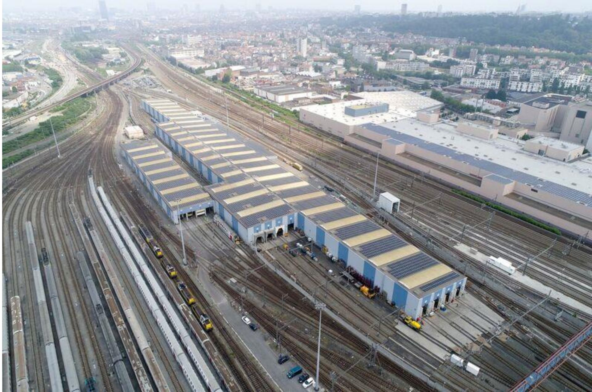
6150 PV panels on the workshop Vorst (Brussel-south) (1,85 MWp)
