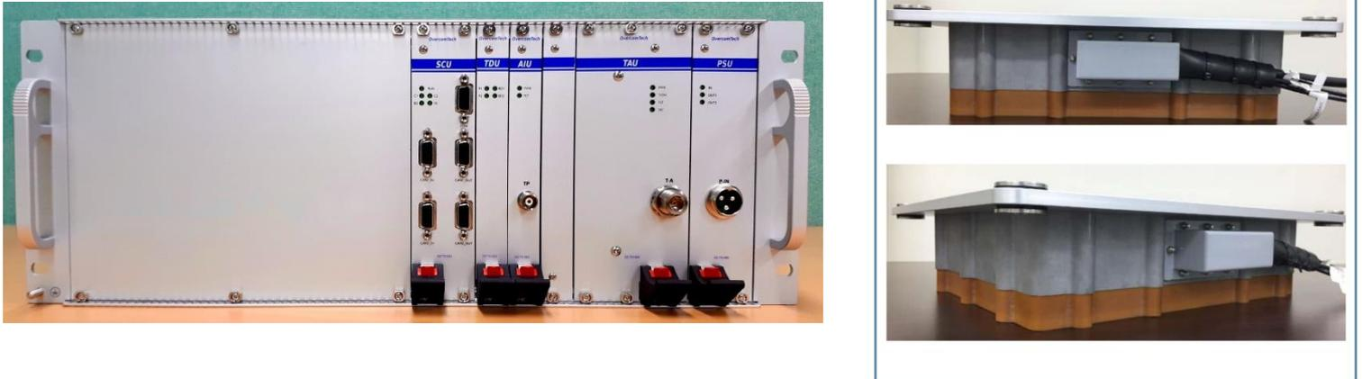
**Figure 8** BTM Module (left) and Antenna (right)
