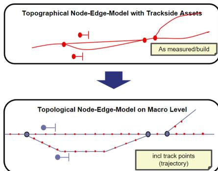
Figure 3 Topological and topographical node-edge-model
