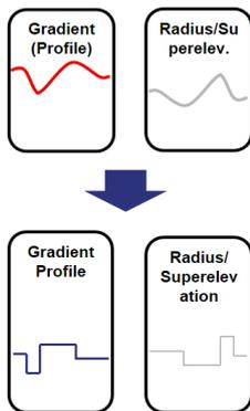
Figure 4 simplification of gradients, radius and superelevation
