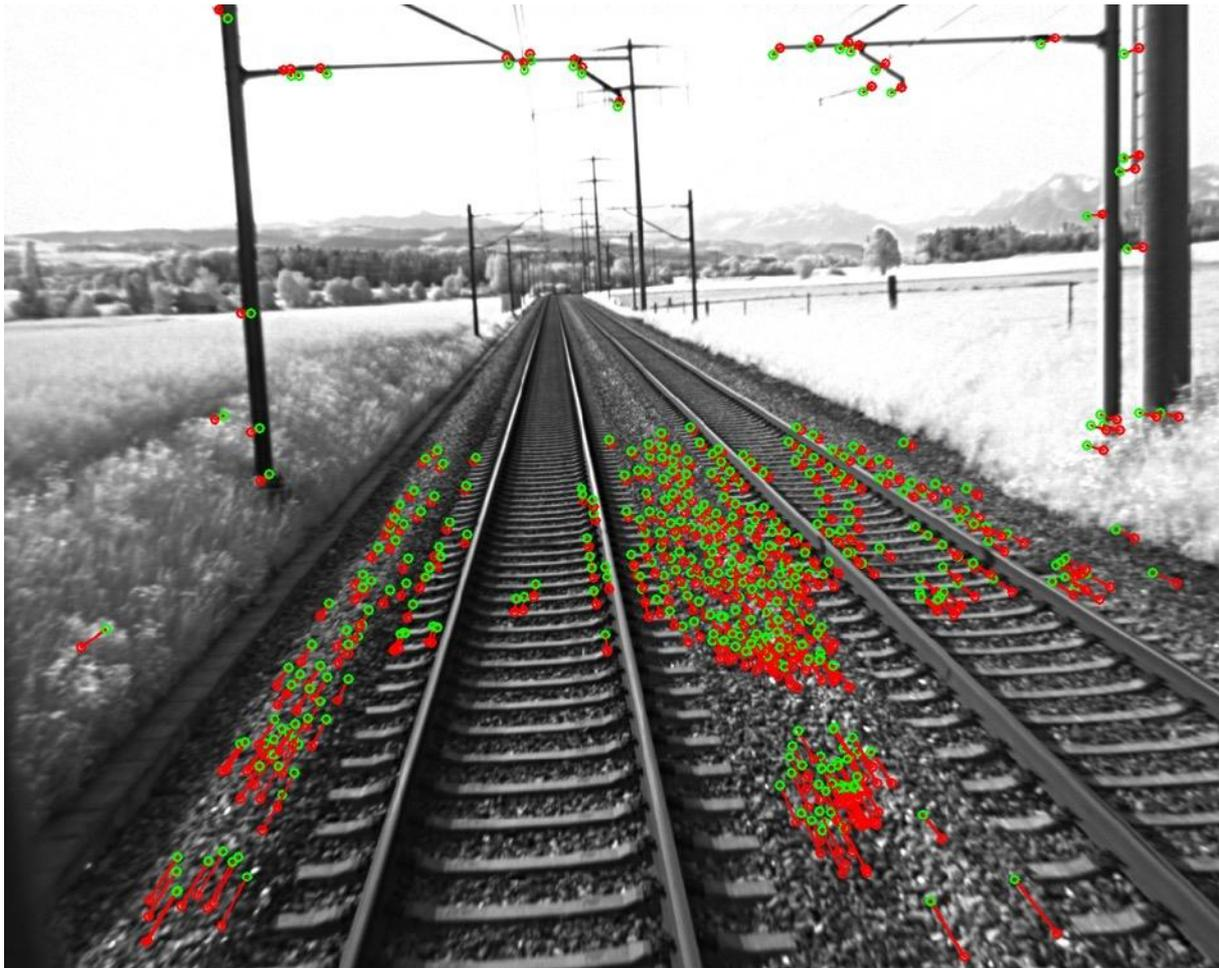
**Figure 3-34: The features of the image are tracked between consecutive frames. Green circles are the features of the previous frame propagated to the next frame (red circles). The apparent motion of the features is displayed as a red line.**
