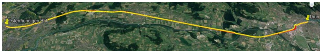
**Figure 6-16** The position calculated with the Visual Odometry (yellow) is corrected by using global reference like railway points and compared to GTG (red).
