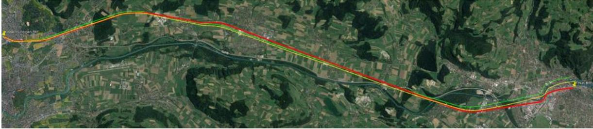
**Figure 3-35:** The train position is calculated over the entire path from Ostermundigen to Thun. The position from GNSS (red) is considered as the reference and compared to the train position calculated in consecutive frames (green). In yellow, the position of the train is calculated by means of keyframes.
