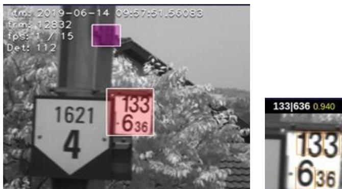
**Figure 7-9.** (left) Image from a side camera pointing 45° relative to the direction of travel. The image shows a geo-referenced mast with a detected kilometer panel (red box) and a detected mast board (purple box). (right) Detected kilometer panel used for OCR analysis. The yellow boxes show the detected digits.
