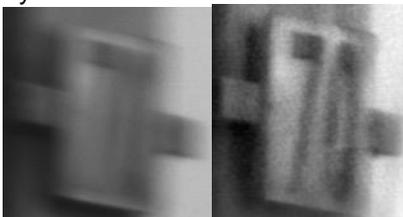
**Figure 7-11.** Example image of mast board with motion blurr (**left**) and after the application of a Wiener Deconvolution filter (**right**).
