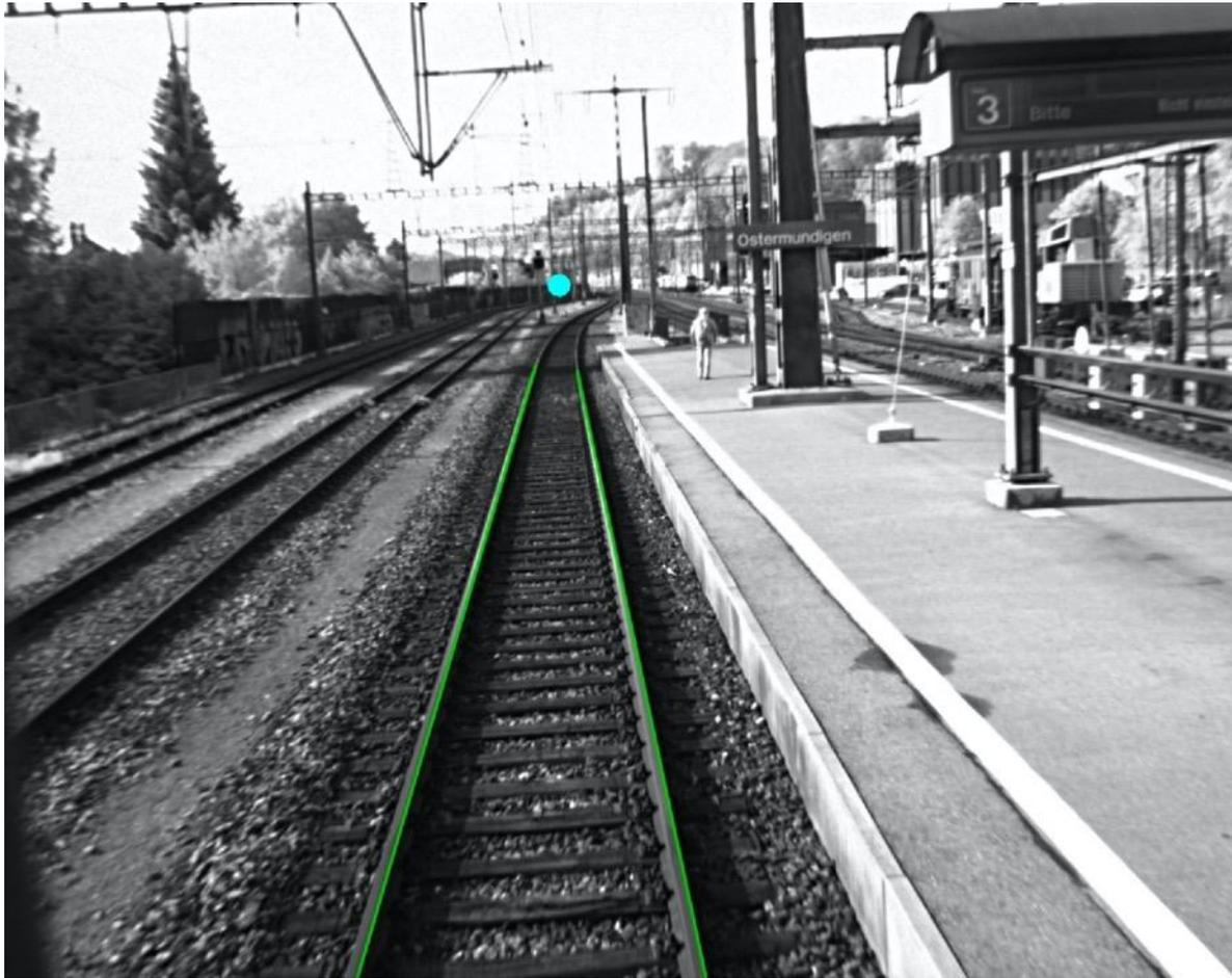
**Figure 3-19: The detected railway track (green) and the vanishing point (cyan) are shown in the image collected.**
