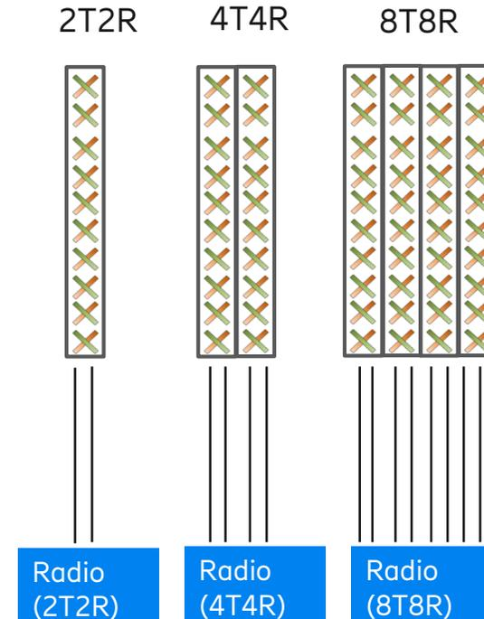
Larger antennas and more feeders are needed for 4T4R and 8T8R
