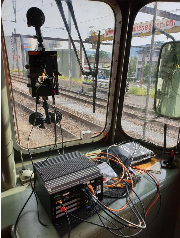
Figure 10-6: The data acquisition system located in the control wagon.
