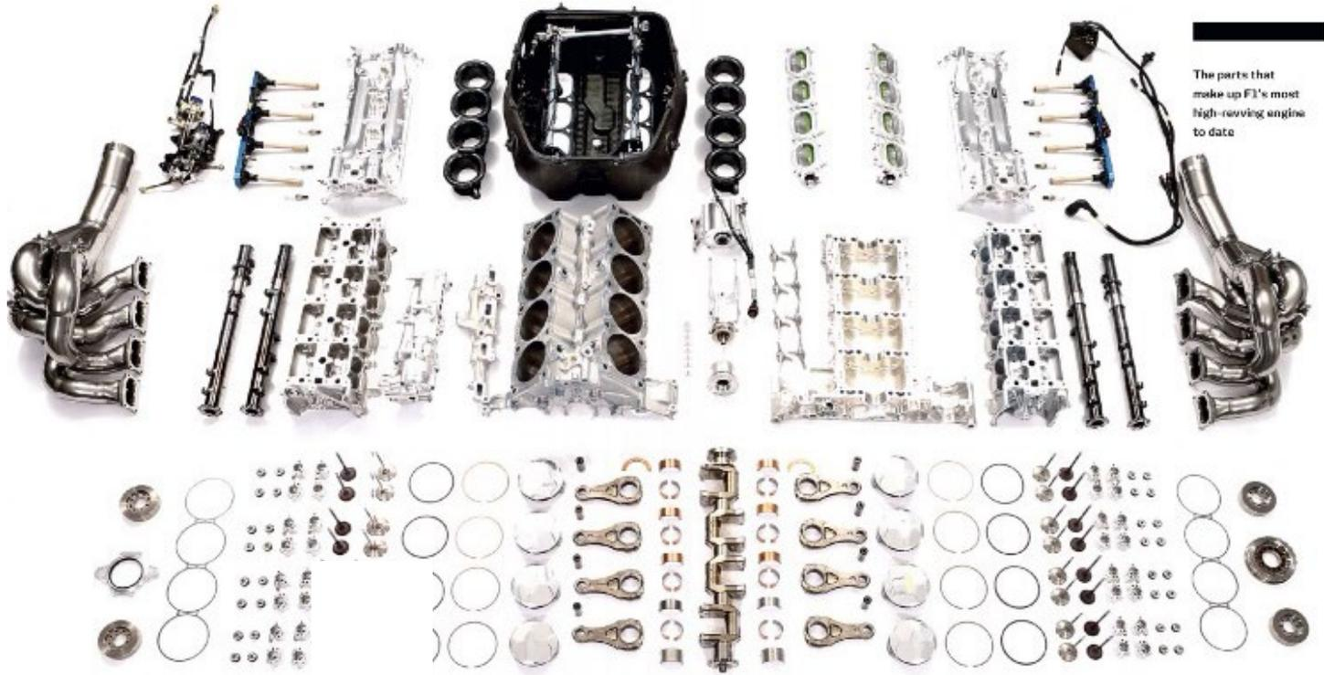
The parts that make up F1's most high-revving engine to date
