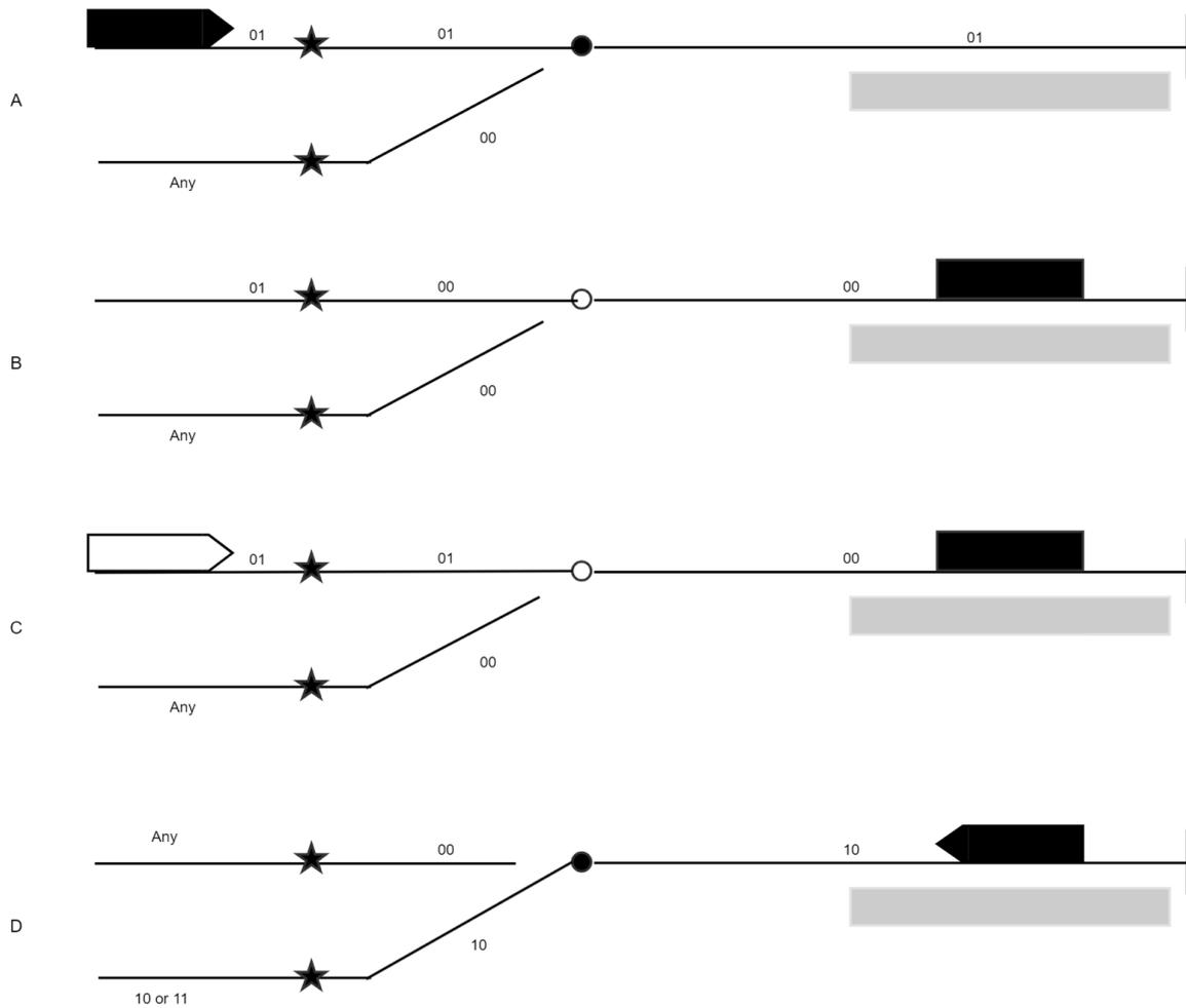
A single terminal platform is a special case where trains must enter and then change direction to exit, often exiting down a different line as depicted in A.
