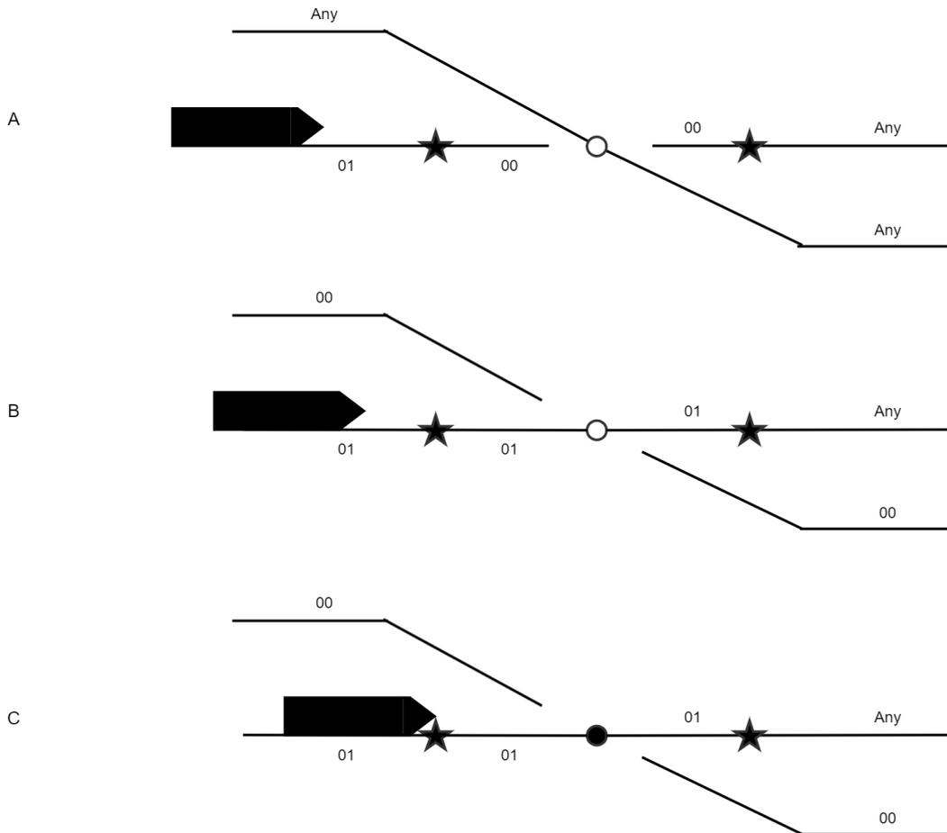
A fixed crossing is treated as a virtual object with 4 edges. The virtual object acts like an instantaneous, and perfectly reliable switch. For a flat crossing placed in plain line, and not near other switches, edge flank protection areas will be required to allow operation. Near other switches or crossings, the need for these would be negated.
