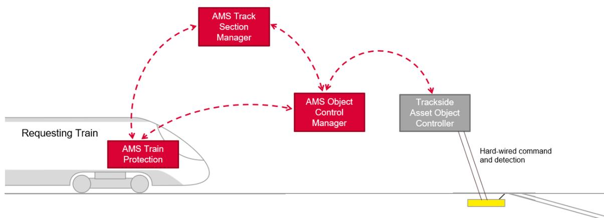
The Trackside Asset Object Controller has a hardware interface with the switch machine and communicates via the AMS Object Control Manager.
