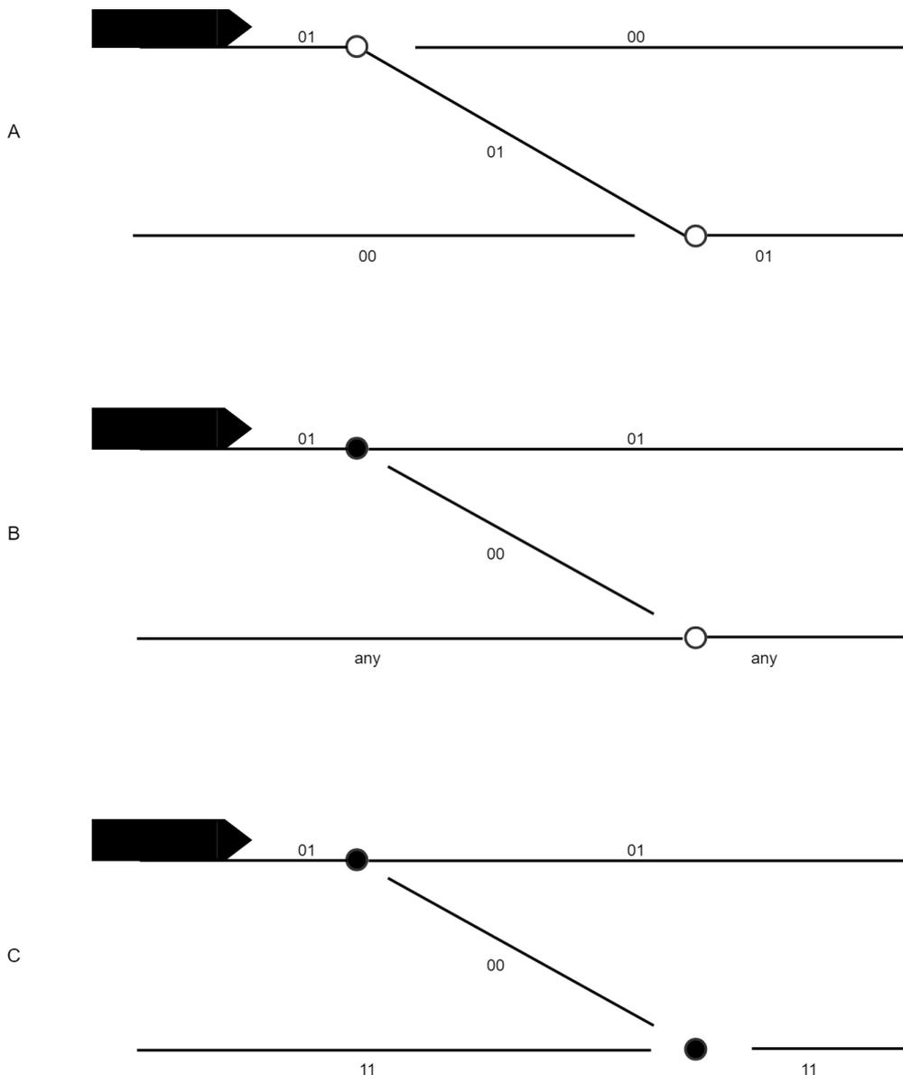
A facing crossover offers a good illustration of the power of edge flank protection area directions to provide passive protection. In A, a train approaches a facing crossover with the goal of continuing straight ahead. The crossover is still set from a previous move. The train requests the reservation of the switch in its path in normal. As none of the switch exit flank directions are locked, the switch complies.
