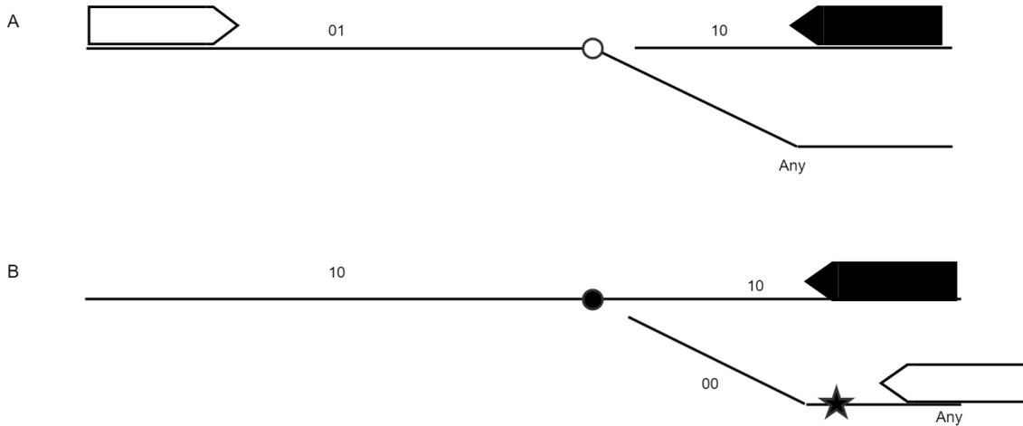
In A, the switch is unreserved, but the edge state on exit is locked due to the presence of the second train, this direction conflicts, therefore the request is denied by the AMS Object Control Manager, thus preventing setting a route which could lead to a collision.
