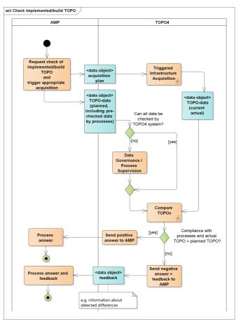
Figure 8 Activity Chart - Check implemented/build TOPO
