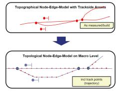
Figure 3 Topological and topographical node-edge-model
