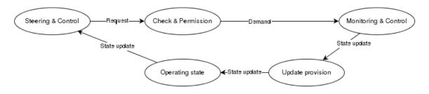
Any request is checked for safety concerns. This check is based on the current operating state and the defined safety rules. Once a request is permitted, it turns into a demand and is transmitted to the physical device for execution. The execution is constantly monitored and controlled. Any state changes are published by the device to the update provision where they are processed and if necessary aggregated to produce a consistent operating state.
