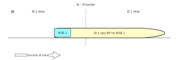
Figure 29 EI 1 sets the by TMS requested MP for MOB 1.
