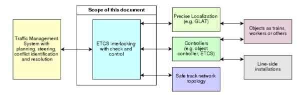
Figure 1 : Schematic description of the smartrail 4.0 system. The scope of this document is the ETCS interlocking.
