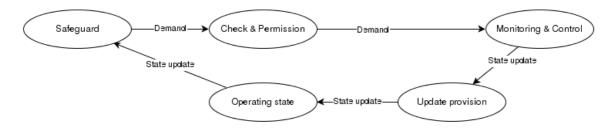
As soon as a safety concern is detected, an emergency safety reaction is performed which results in demands being sent to the domain *Check & Permission* to enter the main processing pipeline.
