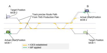
Figure 8 Operating principle MOB, MP – TMS operational disposition
