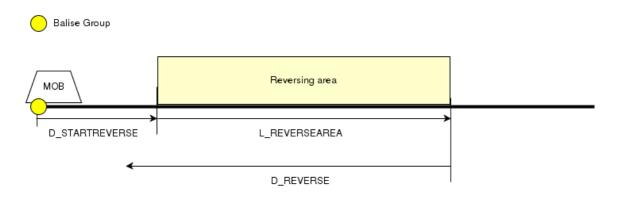
Figure 24 ETCS parameters for reversing.
