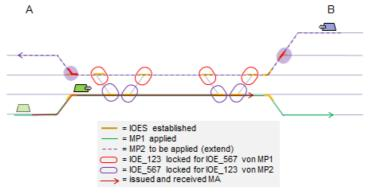
Figure 14 Operating principle MOB, MP - IOESs with reservation and lock protection within an external MP
