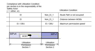
Figure 21 Example of different safety-actors due to geometrical overlap of utilization conditions
