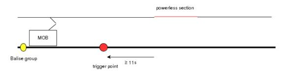
Figure 30 Schematic figure of a powerless section "Switch off main power switch". TMS may not request a MA which ends between the trigger point and the end of the powerless section (note: since the train may not stop inside the powerless section an MP shouldn't end close to the rear of this section).
