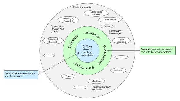
Figure 4 Generic approach of the ETCS interlocking
