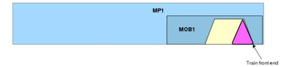
3) The RBC sends the ETCS packets to the train. The RBC itself is responsible, that the train rear end does not leave the MP. Since the reversing distance refers to the train front end the RBC has to guarantee, that the train rear end will remain inside the MP.
