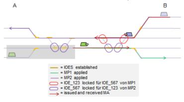
Figure 15 Operating principle MOB, MP - driving and cancellation of protective IOEs
