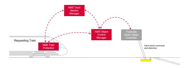
FIGURE 23 - RELATIONSHIP BETWEEN THE ELEMENTS OF SWITCH CONTROL
