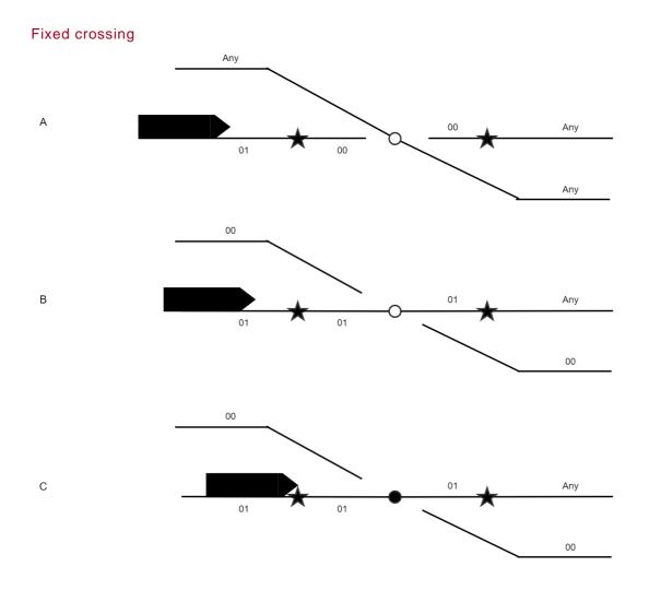
A fixed crossing is treated as a virtual object with 4 edges. The virtual object acts like an instantaneous, and perfectly reliable switch. For a flat crossing placed in plain line, and not near other switches, edge flank protection areas will be required to allow operation. Near other switches or crossings, the need for these would be negated.
