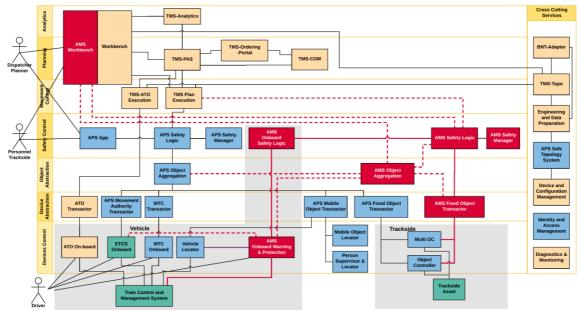
Using an Autonomous Movement Supervision system as a Redundant Safety Layer enables its implementation as software-only, integrated into existing hardware platforms with safety integrity.
