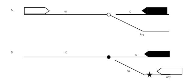
In A, the switch is unreserved, but the edge state on exit is locked due to the presence of the second train, this direction conflicts, therefore the request is denied by the AMS Object Control Manager, thus preventing setting a route which could lead to a collision.
