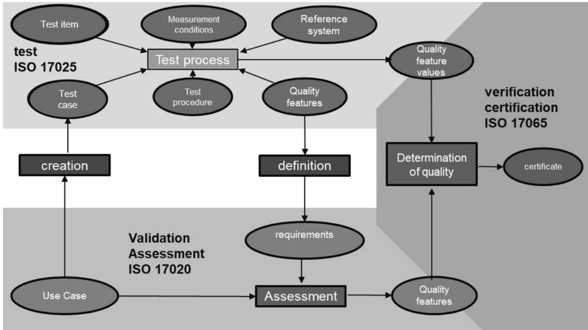
Figure 5-3: Overview: Qualification of a sensor system [27]
