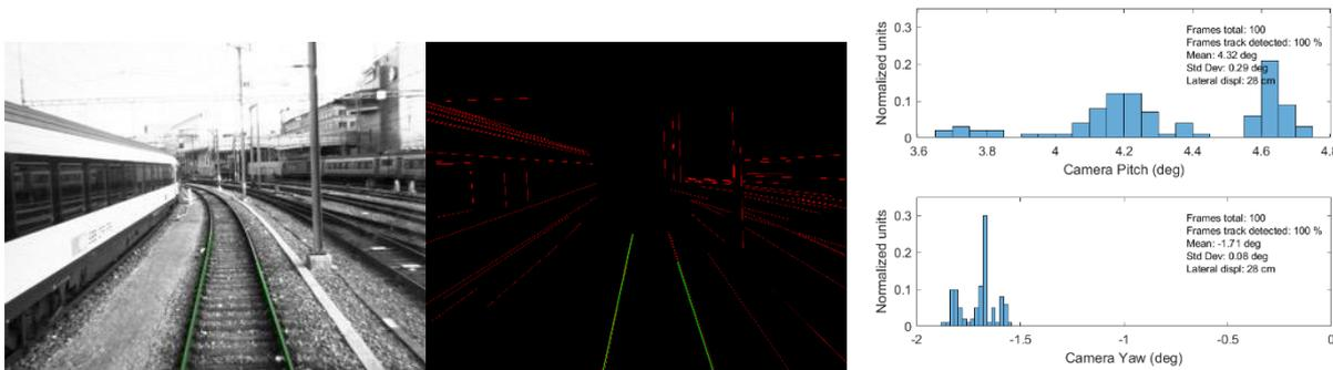
Figure 3-45: Left: Image collected from the camera with identified railway track (green). Middle: Image processed with detected lines (red) and identified railway track (green). Right: Estimated pitch (top) and yaw (bottom) distributions.
