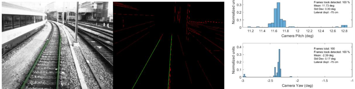
Figure 3-52: Left: Image collected from the camera with identified railway track (green). Middle: Image processed with detected lines (red) and identified railway track (green). Right: Estimated pitch (top) and yaw (bottom) distributions.
