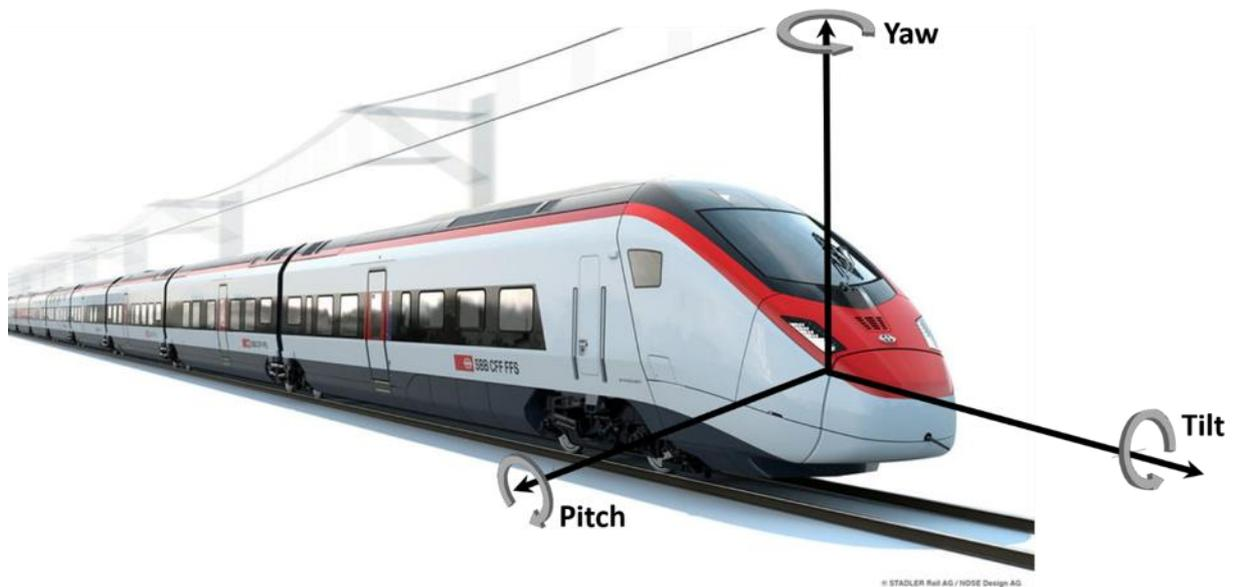
Figure 3-18: Sketch of the Stadler EC250 with the reference system that shows the yaw, pitch and tilt rotations around the axis (Source: <https://bahnblogstelle.net/2017/03/28/stadler-ec250-schweizer-zughersteller-praesentiert-neuen-hochgeschwindigkeitszug-video/>).
