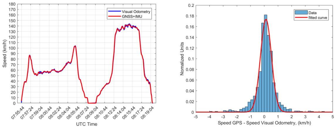
**Figure 6-6 (left)** The absolute speed measured with Visual Odometry (blue) is compared to the one measured with the combination of GNSS and IMU (red) during the drive OT\_2H. **(right)** The distribution of the speed difference between the one measured with GNSS combined with IMU and the one calculated with Visual Odometry is shown for drive OT\_2H.
