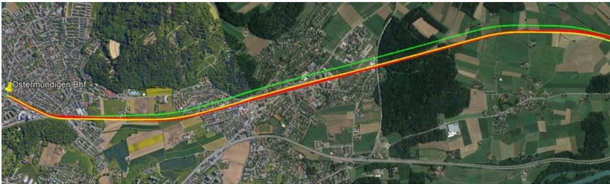
**Figure 3-36:** The train position is shown after few kilometres of the drive from Ostermundigen to Thun. The position from GNSS (red) is considered as the reference and compared to the train position calculated in consecutive frames (green). In yellow, the position of the train is calculated by means of keyframes.
