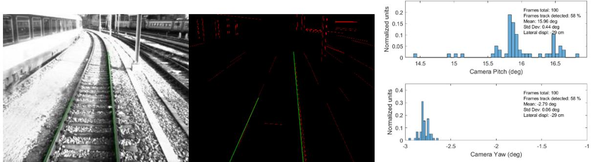
Figure 3-47: Left: Image collected from the camera with identified railway track (green). Middle: Image processed with detected lines (red) and identified railway track (green). Right: Estimated pitch (top) and yaw (bottom) distributions.
