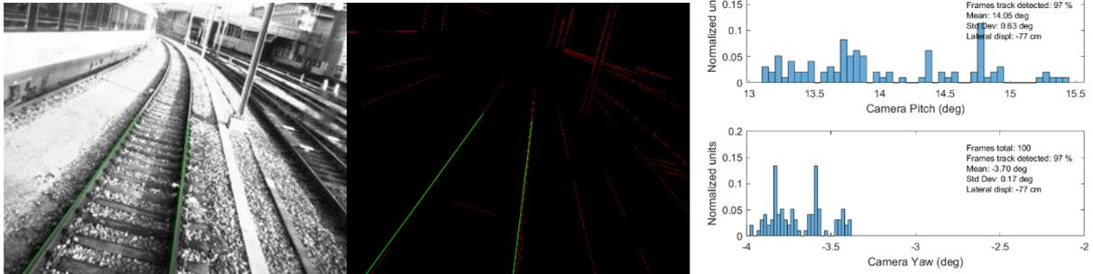
Figure 3-48: Left: Image collected from the camera with identified railway track (green). Middle: Image processed with detected lines (red) and identified railway track (green). Right: Estimated pitch (top) and yaw (bottom) distributions.
