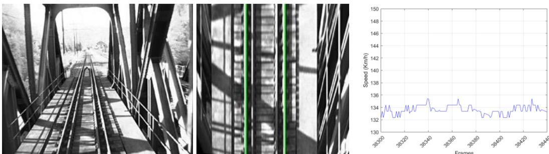
Figure 3-59 (left) Image collected from the camera, where a train is passing the Uttigen bridge, (center) the image transformed to a bird-eye view where the railway track (green) can be identified, (right): the absolute speed is measured with precision meaning that the template matching is not affected by the ground structure of the bridge.
