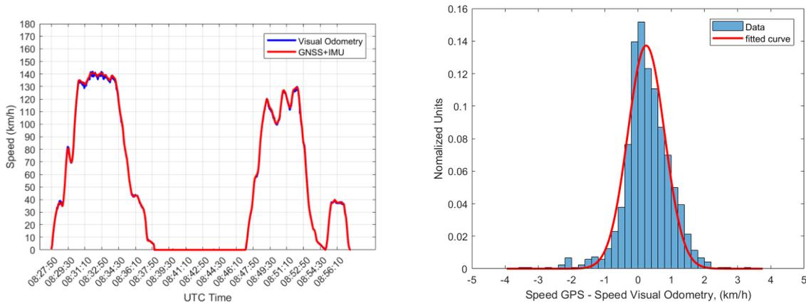
**Figure 6-10 (left)** The absolute speed measured with Visual Odometry (blue) is compared to the one measured with the combination of GNSS and IMU (red) during the drive OT\_2R. **(right)** The distribution of the speed difference between the one measured with GNSS combined with IMU and the one calculated with Visual Odometry is shown for drive OT\_2R.
