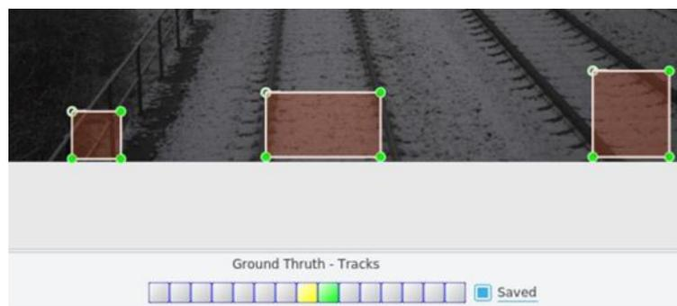
**Figure 7-6.** Example of validated image containing detected tracks (**top**) and “Ground Truth” labels (**bottom**) for visible tracks. The example shows a false positive (FP) detection (left box), where a side-rail is erroneously detected as track.
