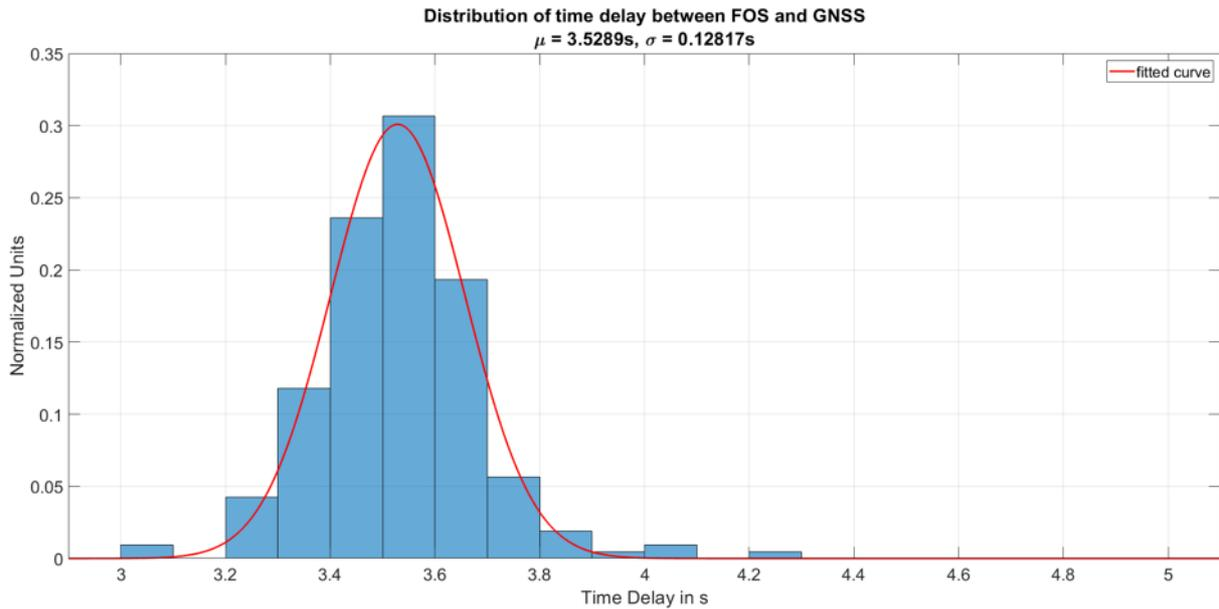
**Figure 6-18 Distribution of the time delay between FOS and GNSS / IMU clock during the drive OT\_1H.**
