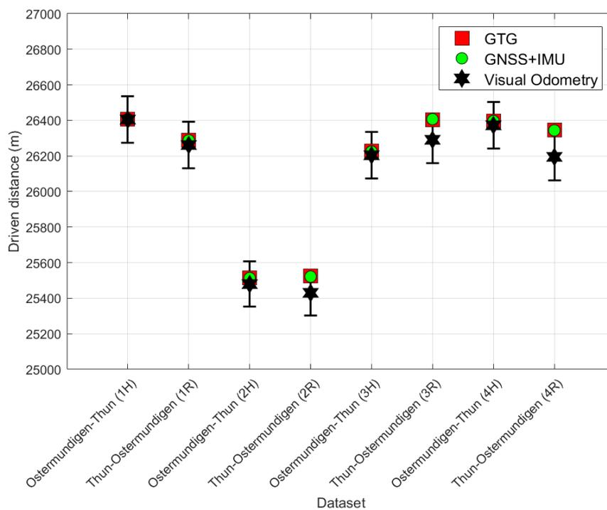
**Figure 6-2: The driven distance is calculated with systematic uncertainty (black) and compared to the GNSS/IMU (green) and GTG (red) measurements.**
