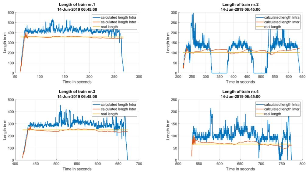
**Figure 4-51** The calculated train length compared to the real length. In blue the train length after the Intra Channel Analysis, in red the corrected train length after Inter Channel Analysis and in yellow the real length.
