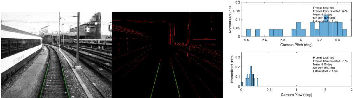
Figure 3-50: Left: Image collected from the camera with identified railway track (green). Middle: Image processed with detected lines (red) and identified railway track (green). Right: Estimated pitch (top) and yaw (bottom) distributions.
