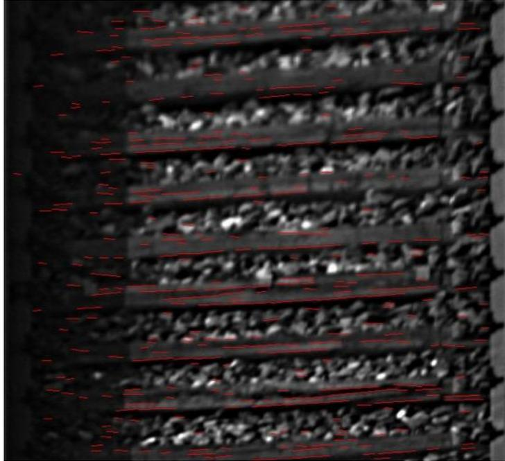
**Figure 3-20:** A bird-eye view of the railway track is shown. The sleepers (red segments) are difficult to be identified by the fast line detector algorithm.
