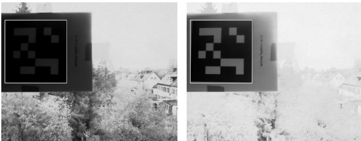
**Figure 3-10 (Left) Image taken using the AES with default brightness reference value. The region of interest is too dark. (Right) Image taken using the AES with calculated brightness reference value. The exposure of the region of interest is sufficient.**
