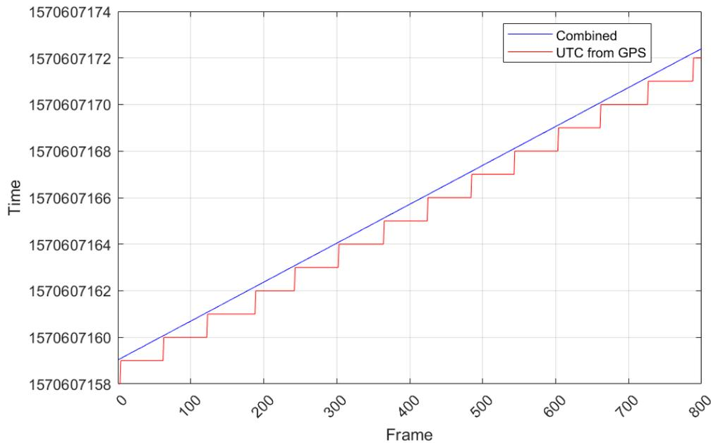
**Figure 3-13** The UTC time from GPS (resolution of 1 second) is compared with the combined time (resolution 1 nanosecond).
