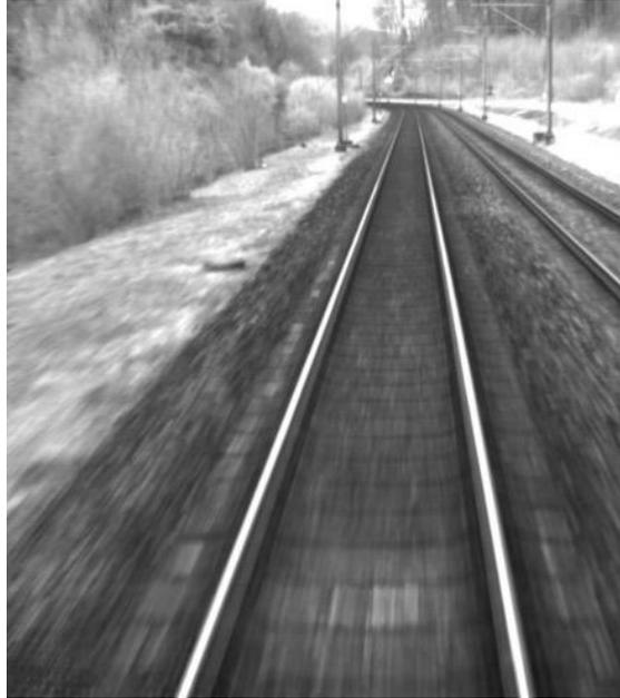
**Figure 3-8** Image collected from a drive from St. Gallen to Bern on a cloudy day in winter. Due to the poor illumination of the scene, the exposure time was automatically set to a high value that causes motion blur resulting in an unsharp image.
