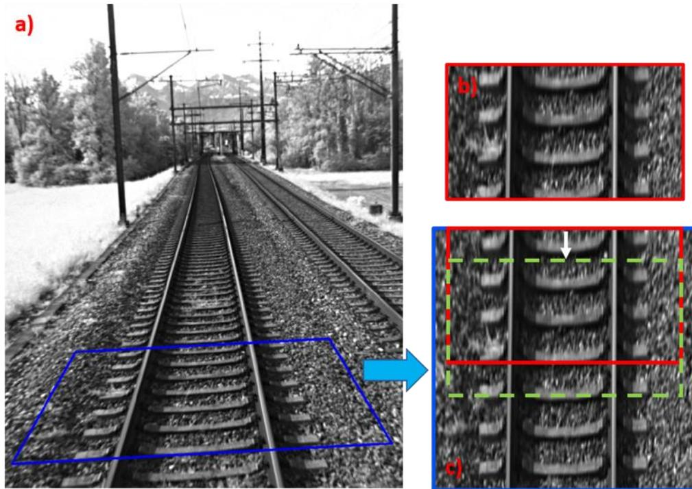
Figure 3-29 a) A search window (blue) is selected in the collected image, b) a template image (from the previous frame), c) the search window is rectified and transformed according to a bird-eye view. The image template b) slides through the search window and the best match is found (green) The pixel displacement (white arrow) between the top of the search image and the position of the green template is proportional to the travelled distance.
