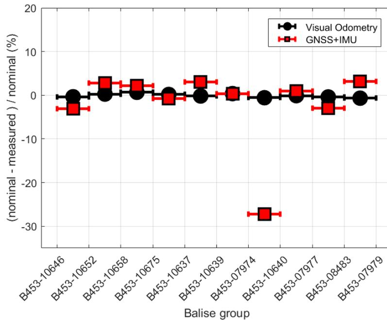
Figure 6-4 The distance between nominal and measured values, divided by the nominal distance is shown. The measured values are from Visual Odometry (red) and from GNSS/IMU (black).
