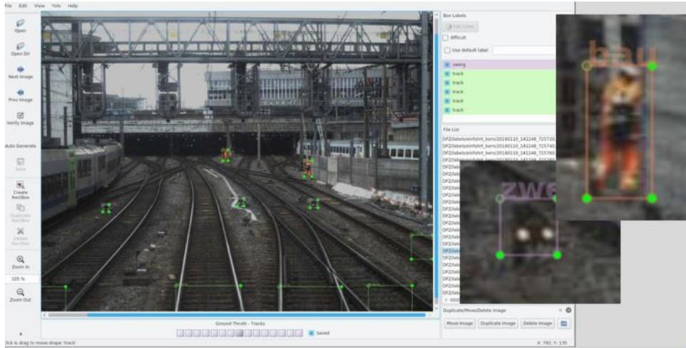
**Figure 7-4.** Adapted interface of the Python based open source tool 'labelImg'. The left image shows an example image extracted from the DFZ. The two images on the right show zoomed in sections of the main image, showing a detected person and “Zwergsignal”, in order to draw the object bounding boxes more precise.
