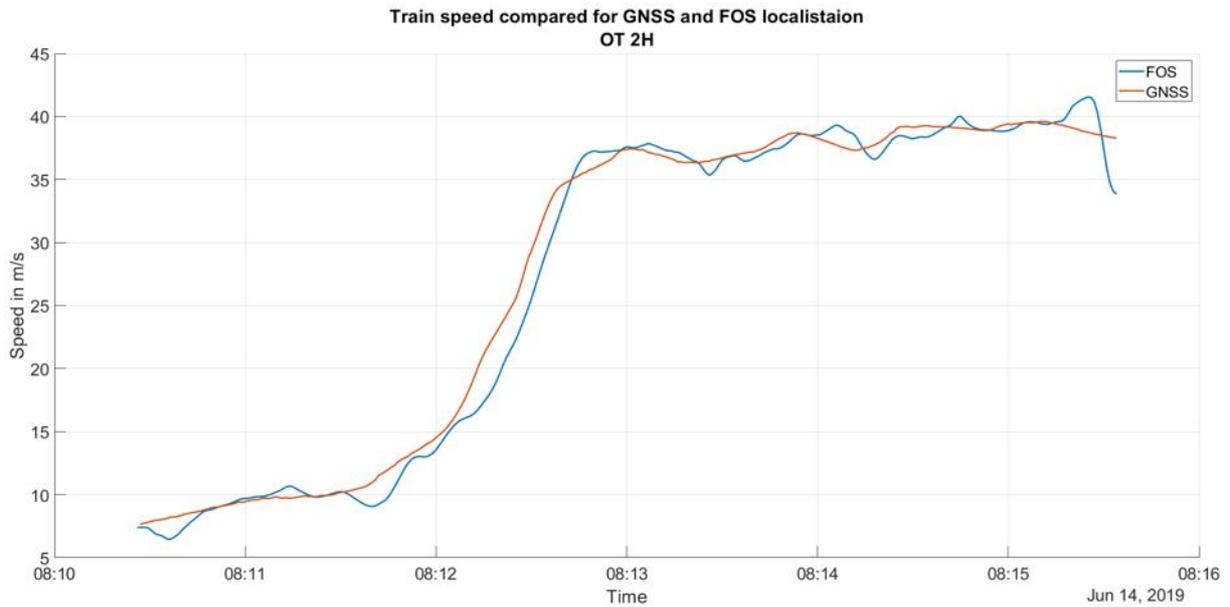
Figure 6-21 Train speed compared for GNSS / IMU and FOS for OT\_2H drive with the measurement train.
