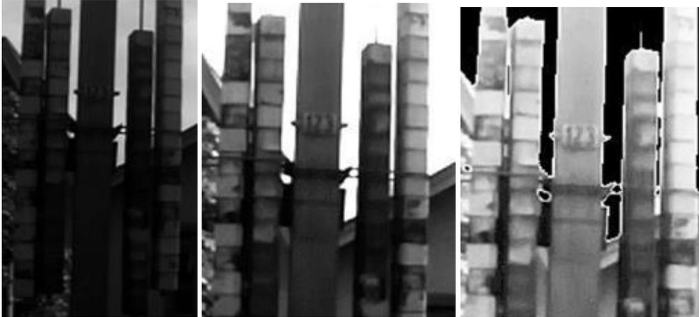
**Figure 7-10.** Example image from mast with extreme image contrast (**left**). Effect of gamma correction on example image (**middle**). Effect of brightness and masked histograms on image gamma corrected image(**right**).
