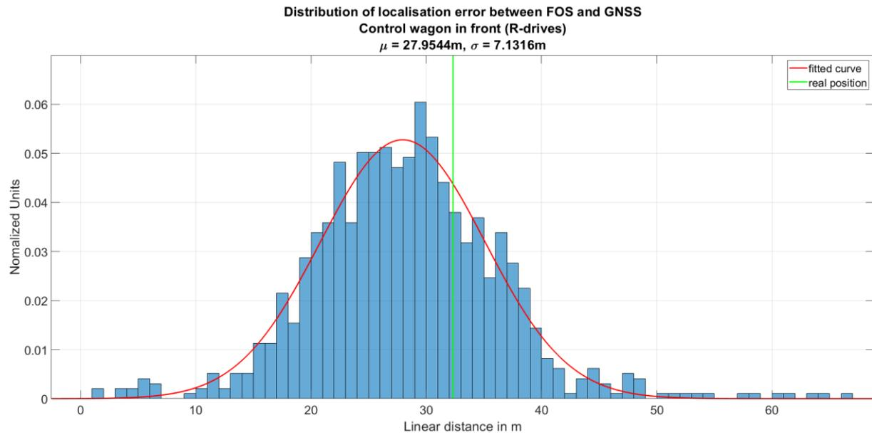
**Figure 6-20** Distribution of the localisation error between GNSS / IMU and FOS for all drives with the control wagon in front position using the front position estimated by FOS. The mean value of the gaussian fit is an estimation of the GNSS / IMU antenna position. Their position is known to be 32.32m behind the front of the control wagon.
