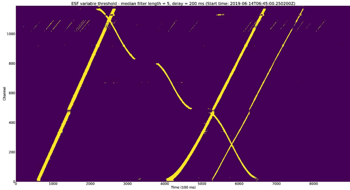
Figure 4-28: ESF threshold based on clustering
