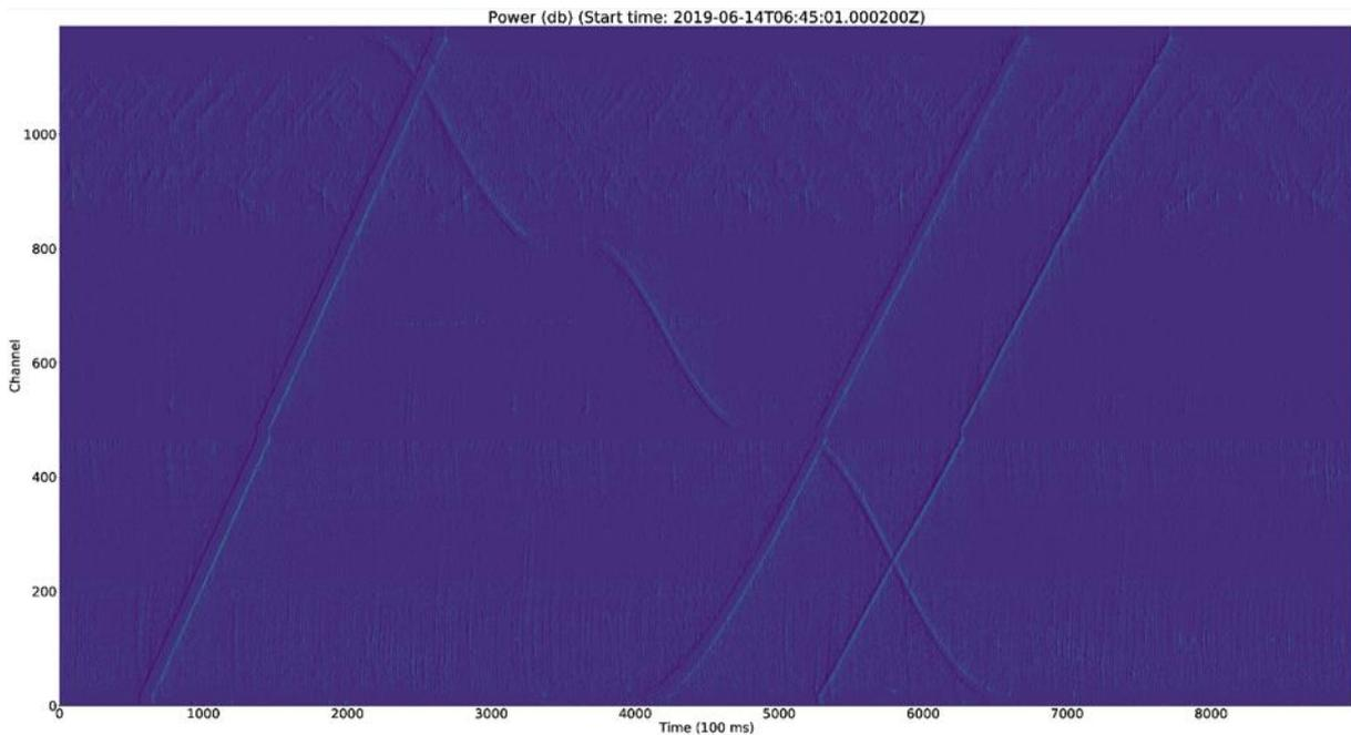
**Figure 4-12: Difference between the DC notch filtered 2500 sample (1 sec) and the 500 sample (0.2 sec) window**
