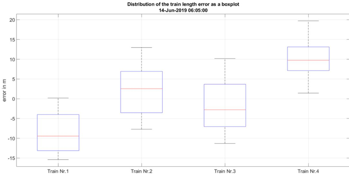
**Figure 4-52** Boxplot showing the distribution of the train length error for all four trains. The initialization phase was excluded because there the train is not fully present in the measurement area.
