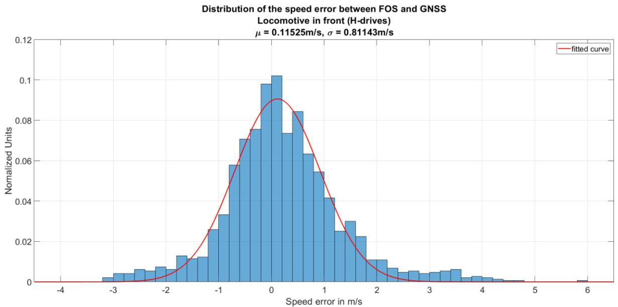
Figure 6-22 Distribution of the speed error between GNSS / IMU and FOS for the drives with the locomotive in the front position.
