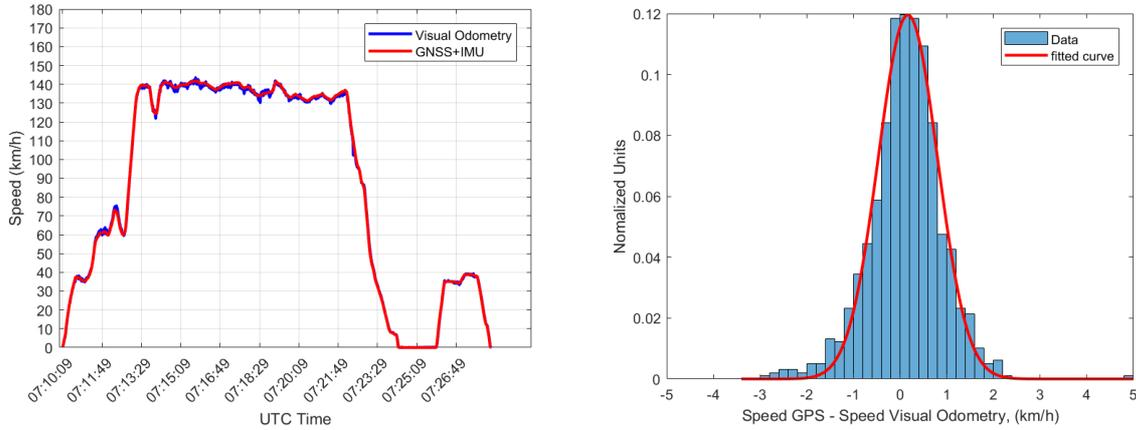
**Figure 6-9 (left)** The absolute speed measured with Visual Odometry (blue) is compared to the one measured with the combination of GNSS and IMU (red) during the drive OT\_1R. **(right)** The distribution of the speed difference between the one measured with GNSS combined with IMU and the one calculated with Visual Odometry is shown for drive OT\_1R.
