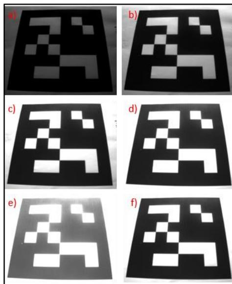
**Figure 3-9** Images with very low illumination (50 lux) at fixed exposure time (16.7 ms). Different gain factors are applied: a) no gain, b) manually set to 33%, c) manually set to 66%, d) manually set to 99%, e) manually set to 99% and gain boost active, f) set to 84% by the automatic gain control.
