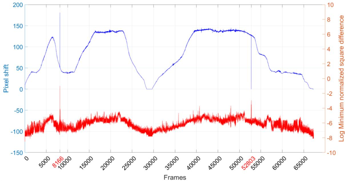
**Figure 3-37** The pixel shift of the template in consecutive frames is shown (blue). The quality of the template matching is evaluated by the value of the minimum of the normalized sum of square differences (red). The template matching in frames 8166 and 52803 failed since the minimum of the normalized sum of square difference was too high.
