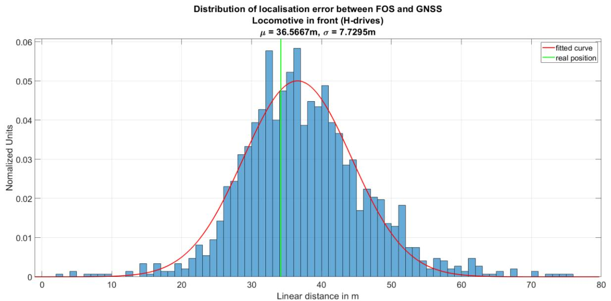
**Figure 6-19** Distribution of the localisation error between GNSS / IMU and FOS for all drives with the locomotive in front position using the front position estimated by FOS. The mean value of the gaussian fit is an estimation of the GNSS / IMU antenna position. Their position is known to be 34.18m behind the front of the locomotive.
