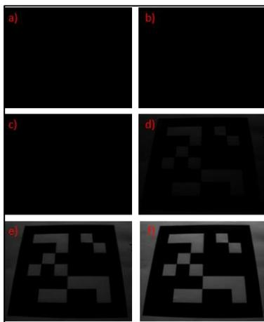
**Figure 3-5** Images with very low illumination (50 lux) with different exposure times:
