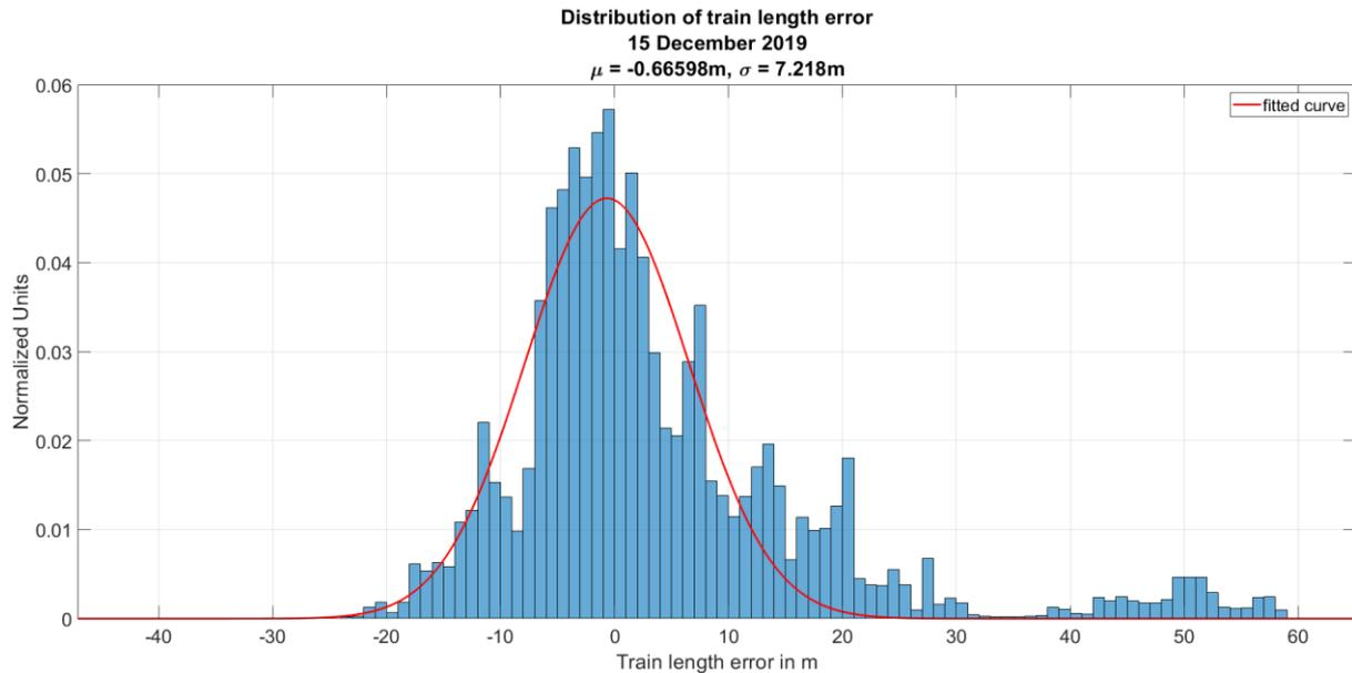
**Figure 4-54** Distribution of the train length error for all trains measured on 15 December 2019. The gaussian fit calculated a nearly zero mean distribution with a precision of 7.218m.
