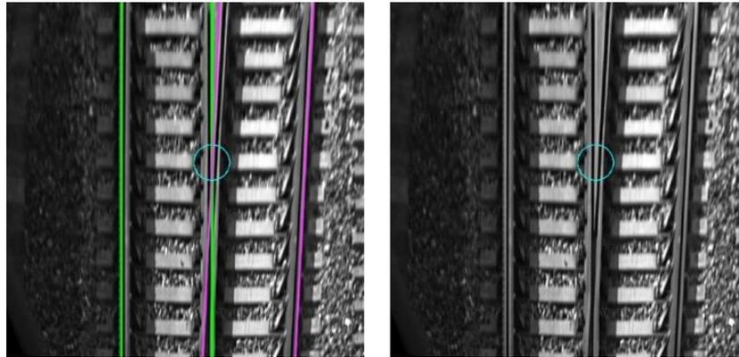
Figure 3-25 Left: The point-frog (circle) is identified from the intersection of the main track (green) and the side track (magenta). Right: A small deviation (~1 meter) between the identified and the truth point-frog is observed.
