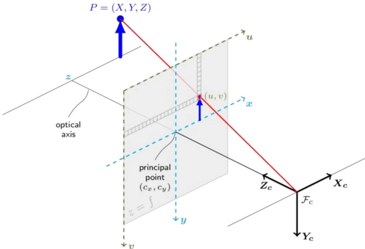
Figure 3-11 The camera pinhole model (Source: [https://docs.opencv.org/2.4/modules/calib3d/doc/camera\\_calibration\\_and\\_3d\\_reconstruction.html](https://docs.opencv.org/2.4/modules/calib3d/doc/camera_calibration_and_3d_reconstruction.html)).
