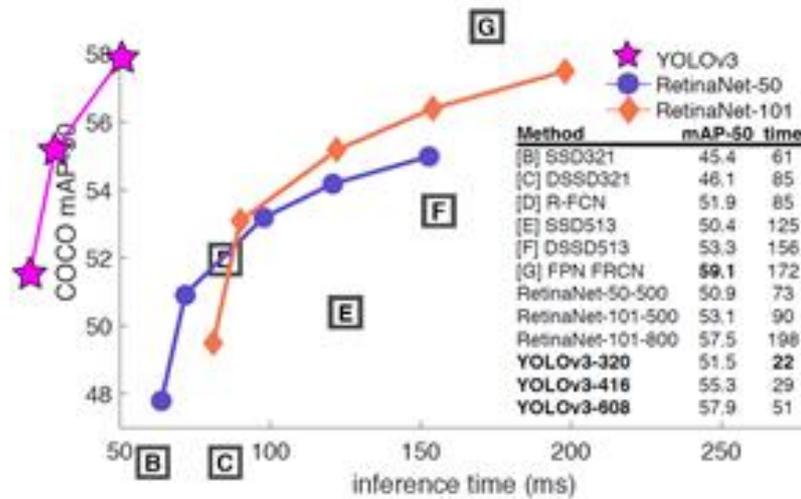
Figure 7-3. Mean average precision (mAP-50, higher is better) shown against the inference time (ms) for different CNN architectures (YOLO framework and different R-CNN frameworks). The mAP-50 is calculated on the COCO object detection dataset from Microsoft.
