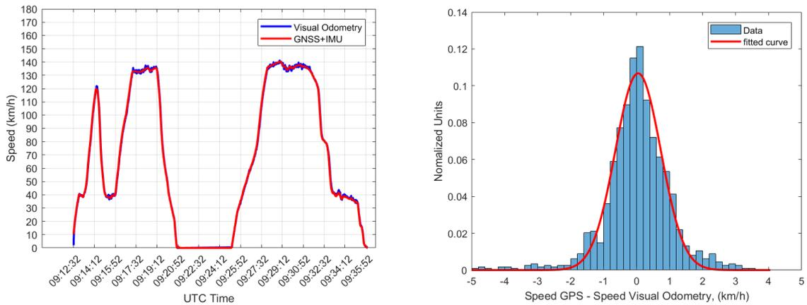
**Figure 6-7 (left)** The absolute speed measured with Visual Odometry (blue) is compared to the one measured with the combination of GNSS and IMU (red) during the drive OT\_3H. **(right)** The distribution of the speed difference between the one measured with GNSS combined with IMU and the one calculated with Visual Odometry is shown for drive OT\_3H.
