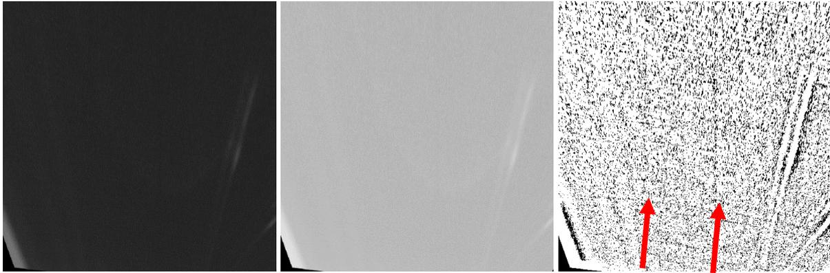
**Figure 3-54:** Left: The collected image is converted from 10 to 8 bits linearly. Middle: The collected image is converted from 10 to 8 bits logarithmically. Right: The logarithmically converted image is processed with an adaptive threshold in order to detect the railway tracks. The track lines, pointed from the red arrows, are poorly visible in the image and cannot be detected.
