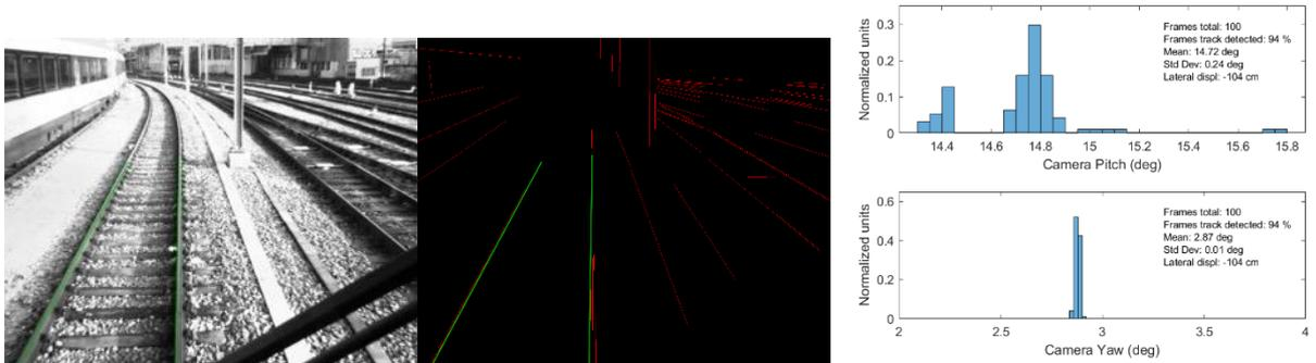
Figure 3-49: Left: Image collected from the camera with identified railway track (green). Middle: Image processed with detected lines (red) and identified railway track (green). Right: Estimated pitch (top) and yaw (bottom) distributions.
