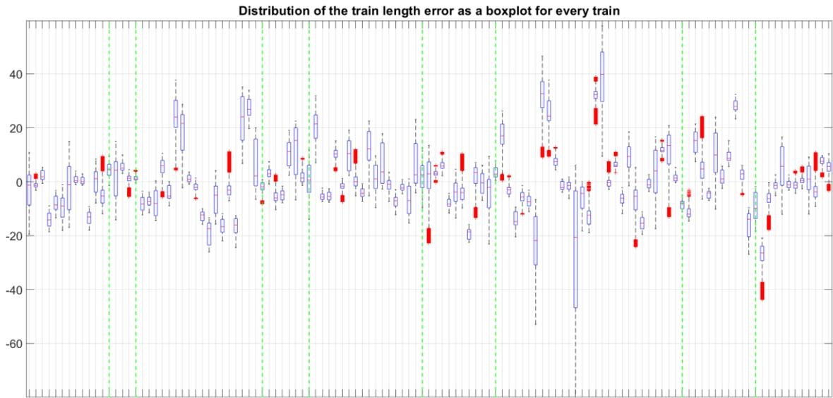
Figure 4-55 Distribution for every tracked train on 14 June 2019 shown as a boxplot. On the x-axis the tracked trains are plotted and on the y-axis the error of true length to calculated length. The measurement train (mewa12) is marked by the dashed green lines.
