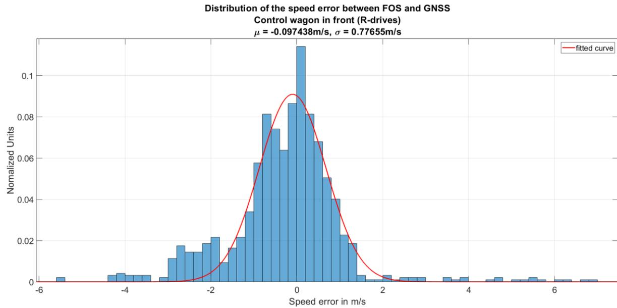
**Figure 6-23** Distribution of the speed error between GNSS / IMU and FOS for the drives with the control wagon in the front position.
