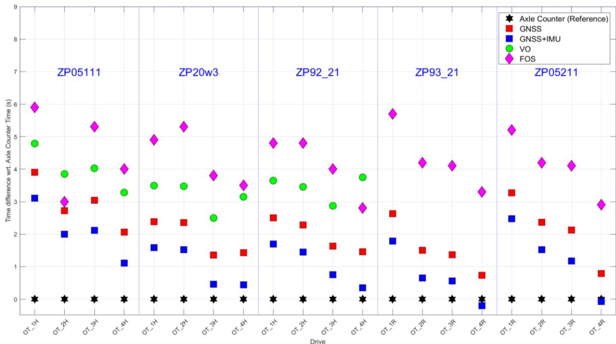
Figure 6-25 Differences in the clocks of the used systems. The axle counter clock is taken as a reference. The figure is divided into blocks which correspond to the axle counter written on the top of each block. On the x-axis the drives are plotted.
