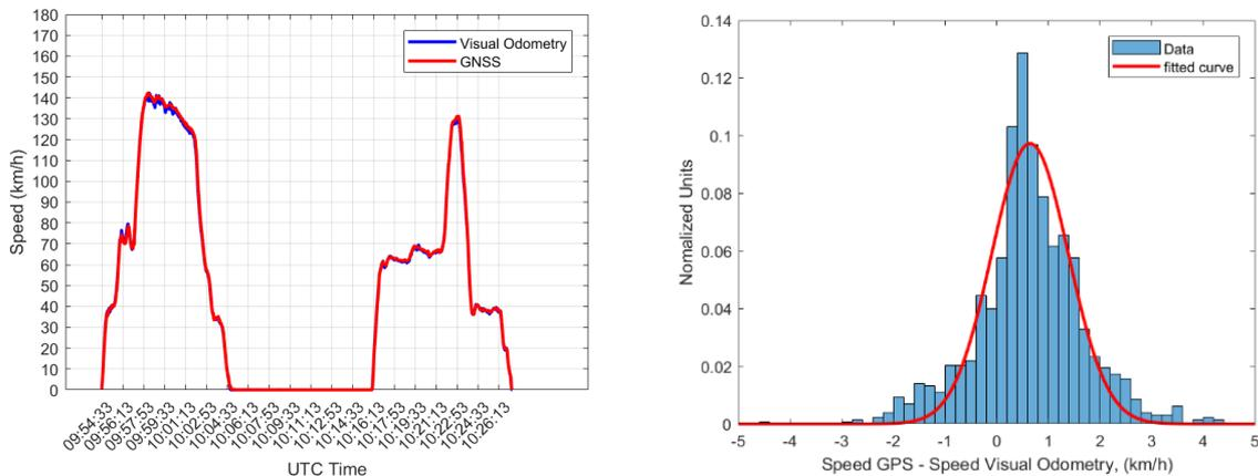
**Figure 6-11 (left)** The absolute speed measured with Visual Odometry (blue) is compared to the one measured with GNSS (red) during the drive OT\_3R. **(right)** The distribution of the speed difference between the one measured with GNSS combined with IMU and the one calculated with Visual Odometry is shown for drive OT\_3R.
