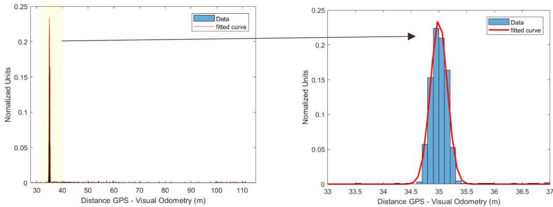
**Figure 6-15** The distribution of the difference between the position measured from GNSS/IMU combination and the one calculated with Visual Odometry by using railway point as reference. The distribution peaks at 35 meters. This is the position of the IMU, that is located 35 meters back with respect to the camera system, that is located at the front of the train. (Left) The distribution ranges from 20 to 150 meters and the tails can be seen. (Right) The distribution ranges from 33 to 37 meters.
