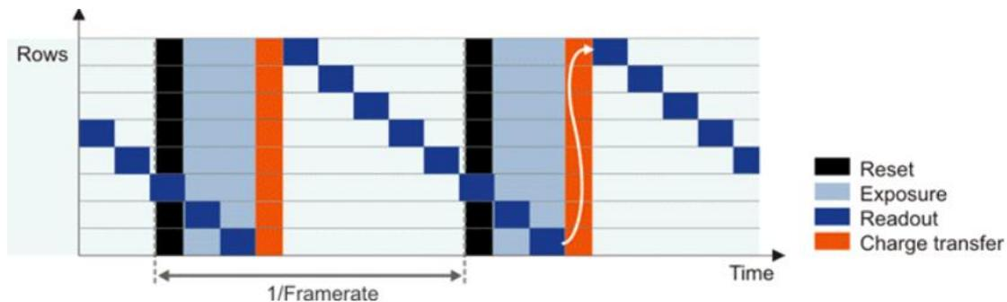
Figure 3-4 Global shutter sensor in live mode (Source: [5]).
