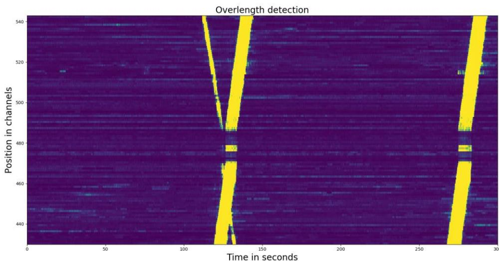
**Figure 4-42** Energy spectrum at station Wichtrach showing the area of the rolled-up fiber.
