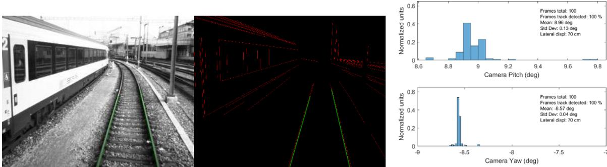
Figure 3-44 Left: Image collected from the camera with identified railway track (green). Middle: Image processed with detected lines (red) and identified railway track (green). Right: Estimated pitch (top) and yaw (bottom) distributions.
