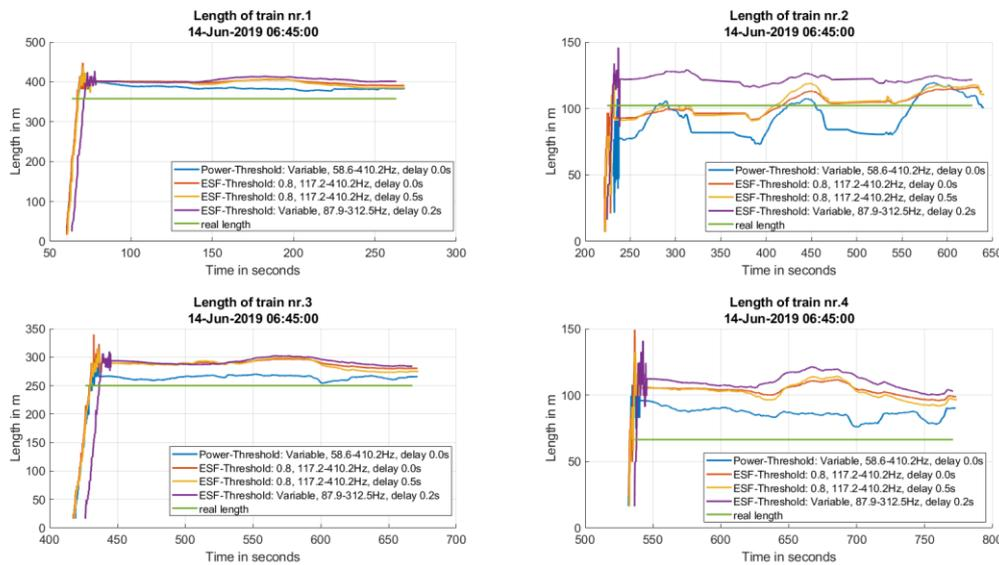
**Figure 4-50** Lengths of the four trains compared for all the settings in the Intra Channel Analysis. Lengths match with Tracking in Figure 4-48:.
