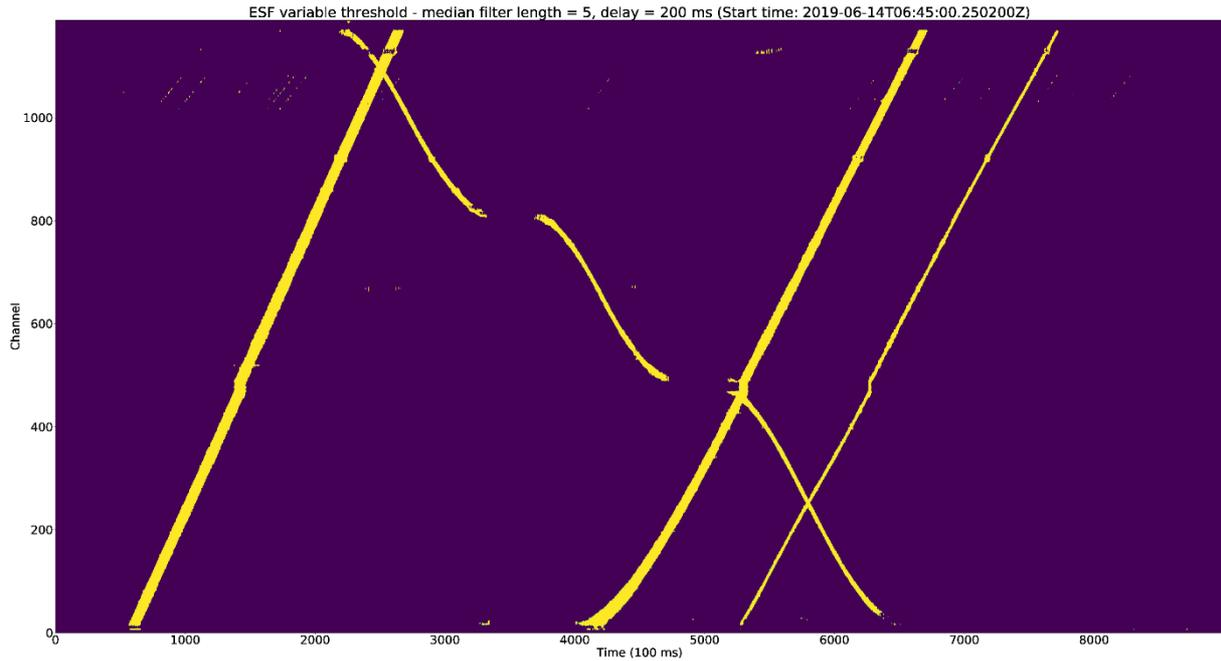
Figure 4-32: ESF threshold based on clustering with variable filtering for the sample 15 minute interval (14 June 2019)
