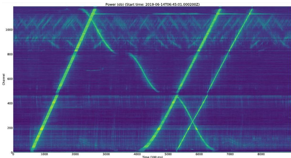
**Figure 4-10: DC notch filtered data power using a 2500 sample (1 sec) window and a 250 sample (0.1 sec) step**
