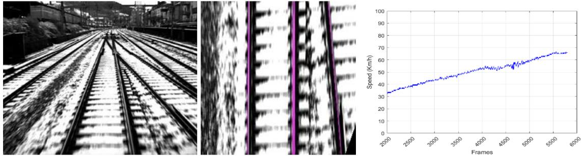
**Figure 3-55 (left):** Image collected from St Gallen to Bern (data from drive BSG\_1R) with snow on the railway track, **(center):** the image is transformed to a bird-eye view where the railway track (magenta) can be identified, **(right):** the absolute speed is measured with precision meaning that the template matching is not affected by the snow.
