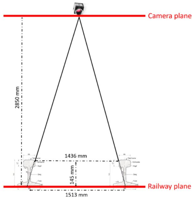
Figure 3-33 The railway track internal width is propagated to the ground, according to the angle of view of a bird-eye image.
