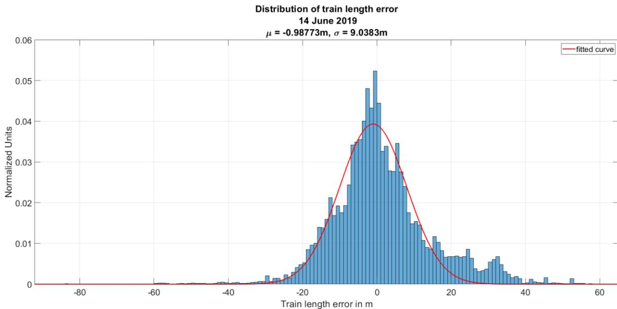
**Figure 4-53 Distribution of the train length error for all trains measured on the 14 June 2019. The gaussian fit calculated a nearly zero mean distribution with a precision of 9.0383m.**
