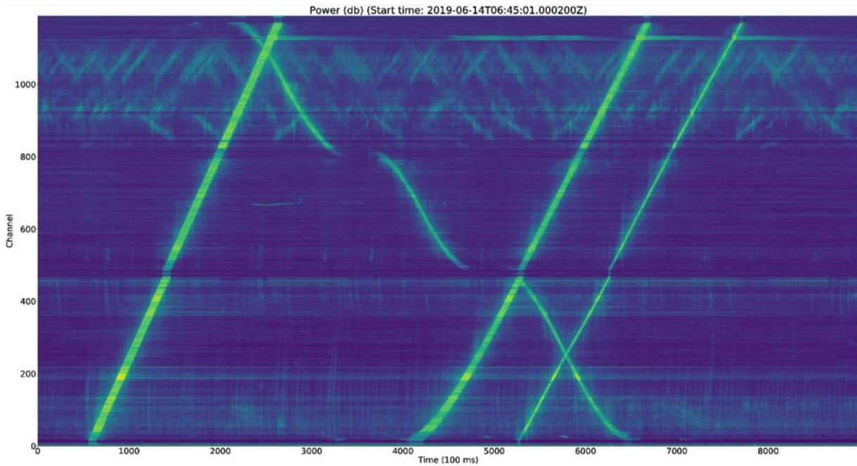
**Figure 4-11: DC notch filtered data power using a 500 sample (0.2 sec) window and a 250 sample (0.1 sec) step**
