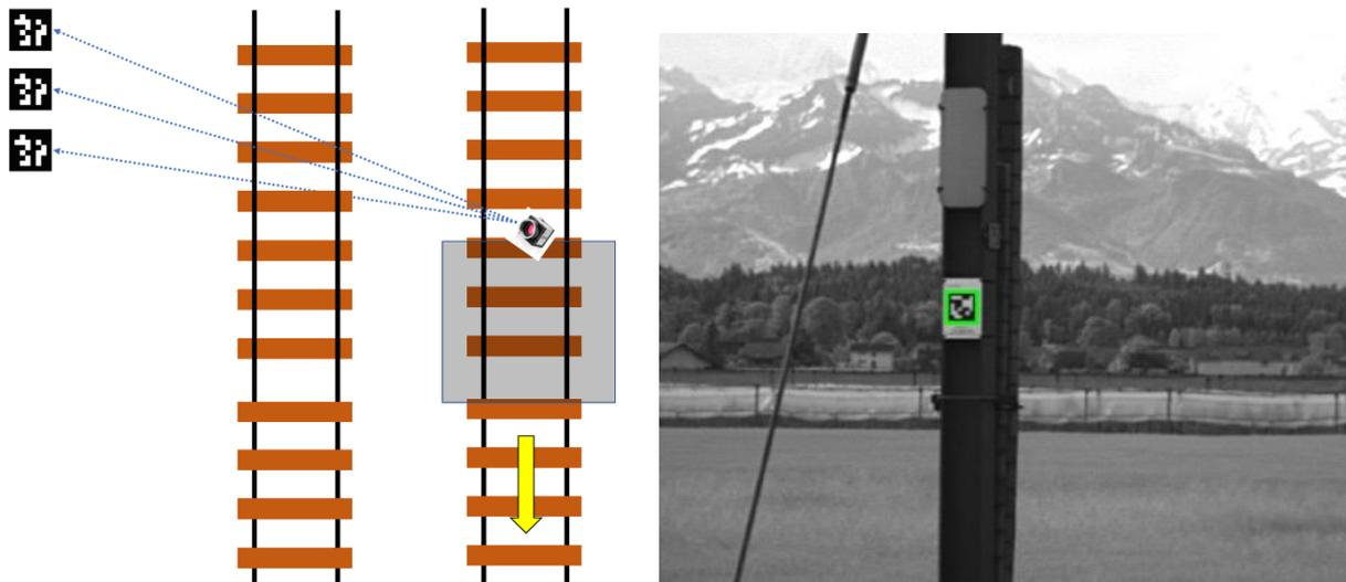
Figure 3-40 Left: scheme of the camera system moving backwards and passing by an AprilTag. Right: image where the AprilTag is detected (green square).
