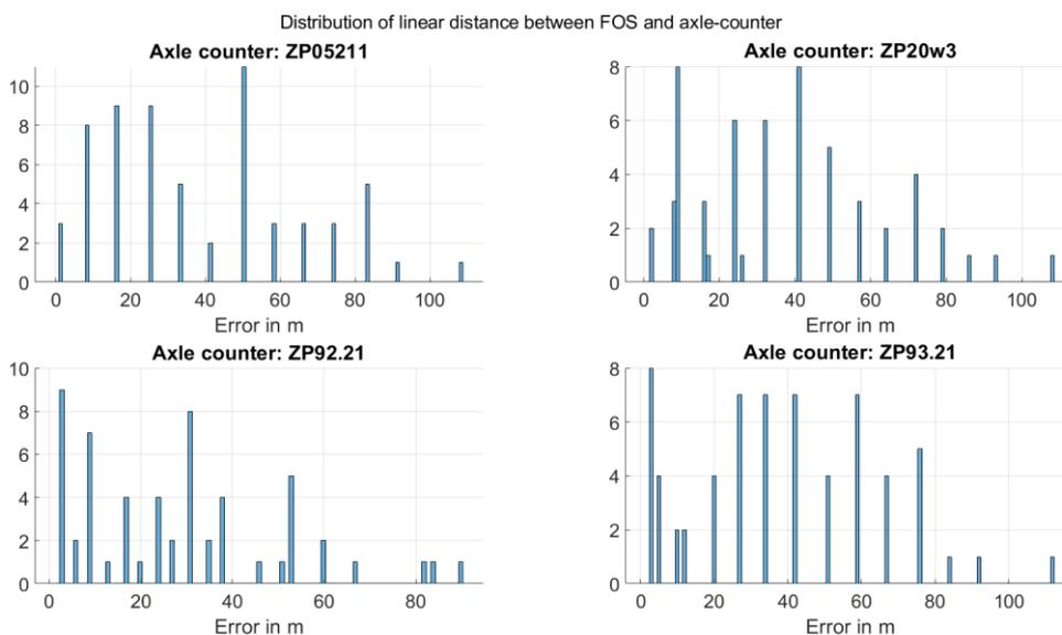
Figure 6-24 Distribution of the localisation error between FOS and axle counters.
