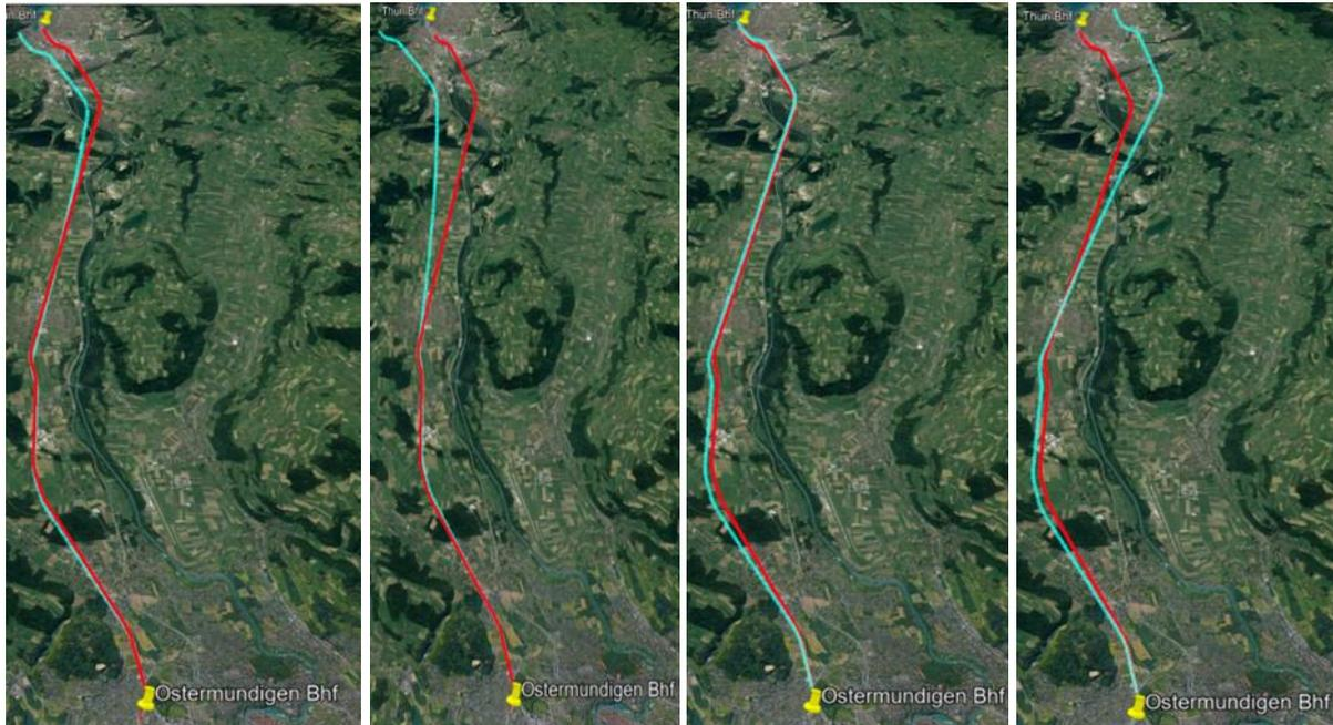
**Figure 6-13: The calculated position (cyan) for the 4 drives (from left to right: OT\_1H, OT\_2H, OT\_3H, OT\_4H) from Ostermundigen to Thun and compared to the GNSS/IMU reference (red)**
