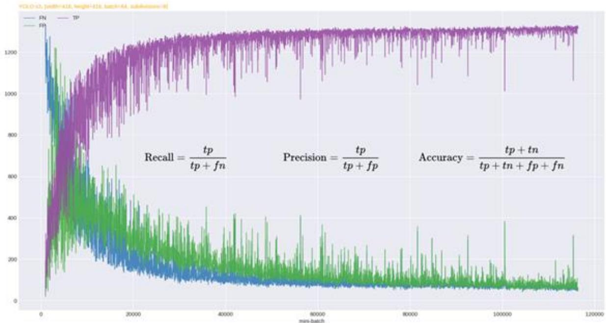
**Figure 7-5.** Development of the values for TP (purple), FP (green) and FN (blue) detections during training. As expected, the TP detections increase, and the FP and FN detection decrease towards a limit during the training process.
