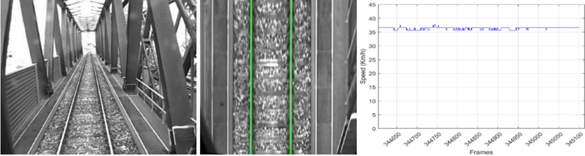
Figure 3-60 (left) Image collected from the camera, where a train is passing the bridge before the Brig station, (center) the image transformed to a bird-eye view where the railway track (green) can be identified, (right): the absolute speed is measured with precision meaning that the template matching is not affected by the ground structure of the bridge.
