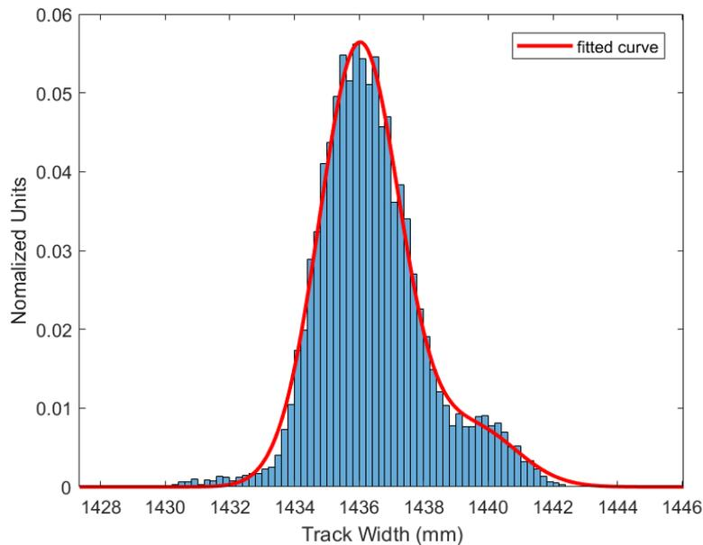
**Figure 3-31: The distribution of the measured track width for run OT\_1H is shown. A double gaussian fit has been performed to extract the mean value and the standard deviation.**
