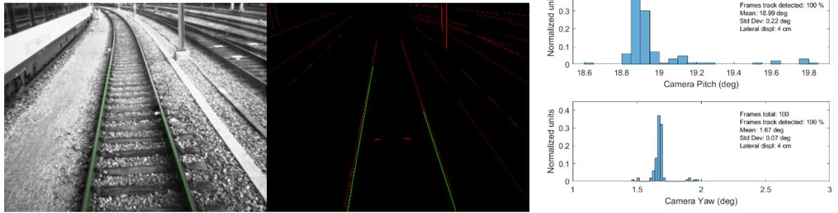
Figure 3-46: Left: Image collected from the camera with identified railway track (green). Middle: Image processed with detected lines (red) and identified railway track (green). Right: Estimated pitch (top) and yaw (bottom) distributions.
