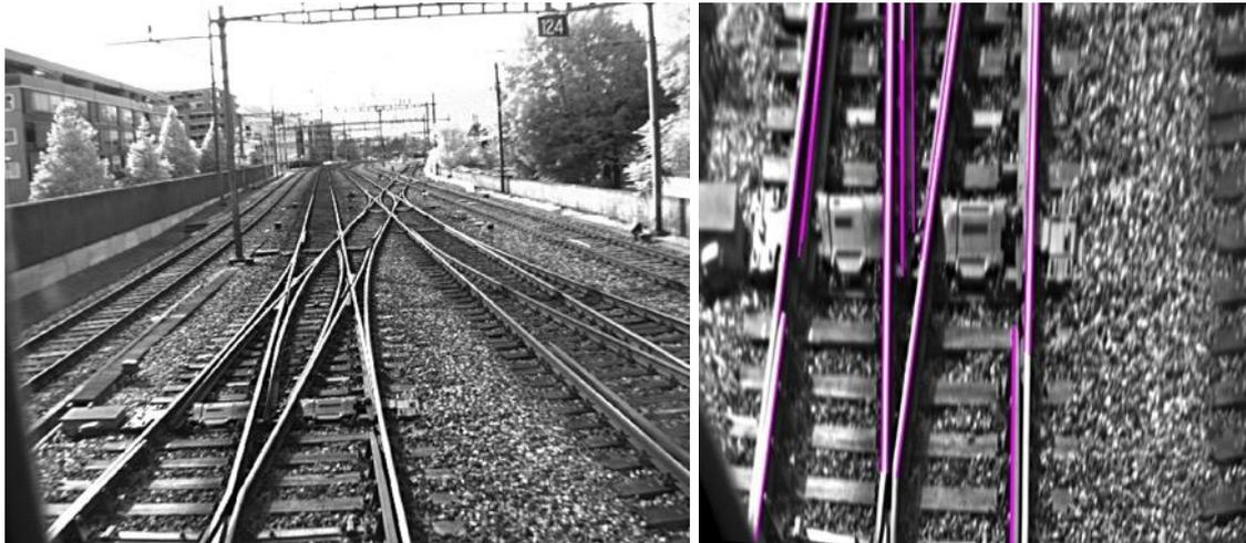
Figure 3-27: (left): The image of a crossing point is collected, (right): A bird-eye view of the crossing point with detected lines (magenta). The tongue rail can be hardly identified among the detected lines.
