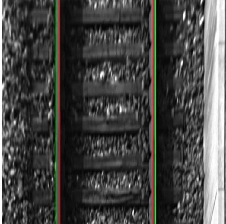
Figure 3-32 The internal (red) and external (green) track profile are identified in the collected image.
