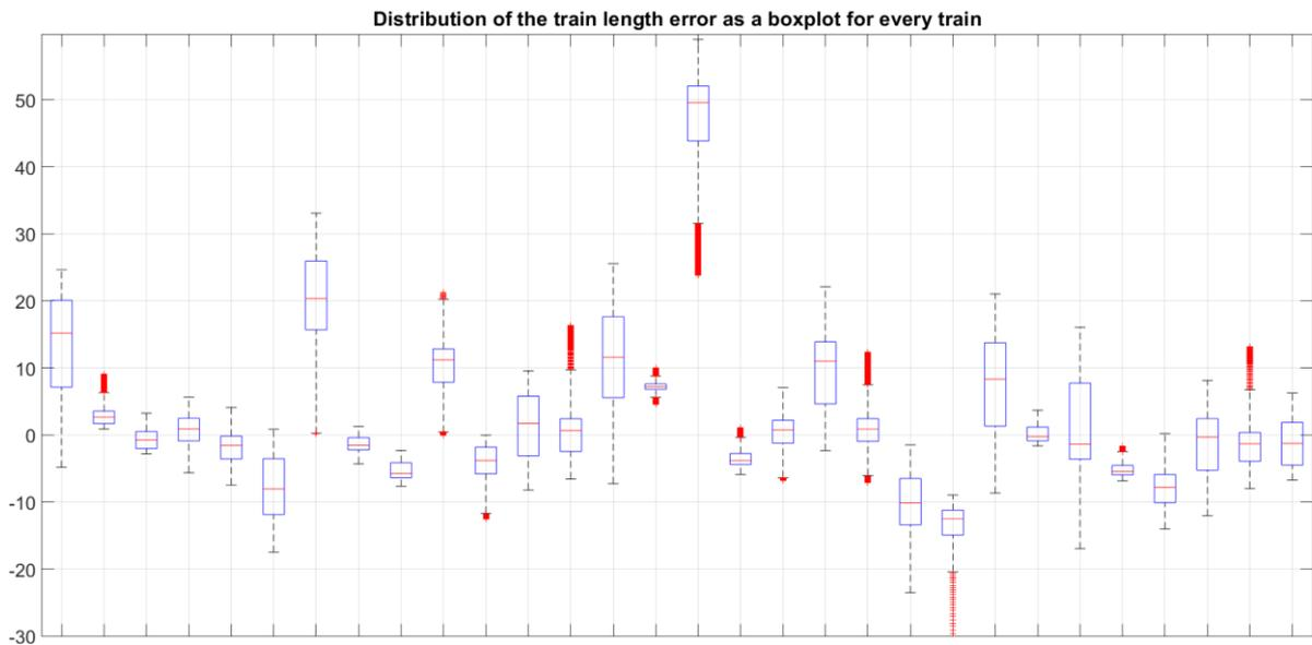
Figure 4-56 Distribution for every tracked train on 15 December 2019 shown as a boxplot. On the x-axis the tracked trains are plotted and on the y-axis the error of true length to calculated length.
