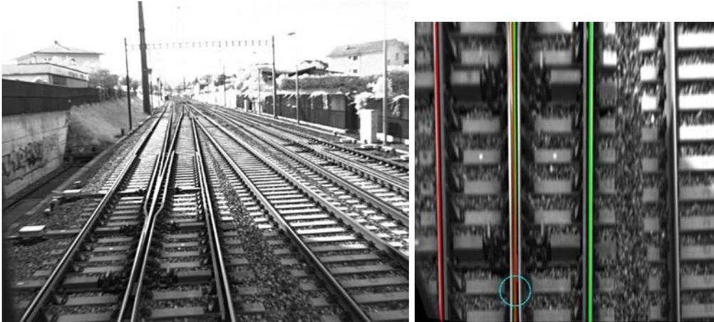
**Figure 3-26 (left):** The image of a high-speed point is collected, **(right):** A bird-eye view of the high-speed point, where both main (red) and side (green) tracks are detected. The tracks are almost parallel and the intersection is difficult to measure.
