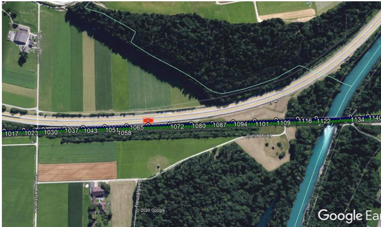
Figure 4-44 Google Earth picture showing the mapping where FOS can be affected by external influences. Cars driving on the highway produce noise and the whole bridge vibrates when a train is passing which makes it more difficult to get a clear front and rear end at this section.
