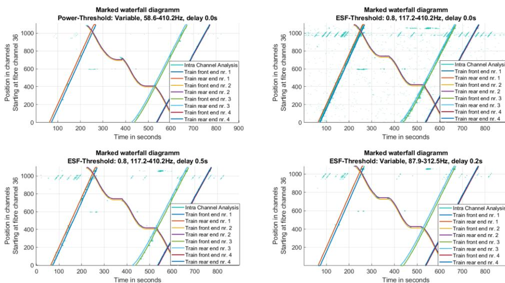
**Figure 4-48: Different approaches and parameters in the Intra Channel Analysis and the calculated tracking of front and rear ends by the Inter Channel Analysis**
