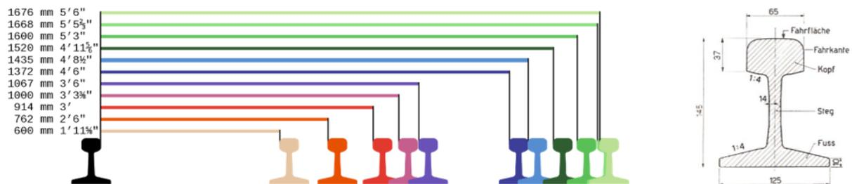
Figure 3-30 (left): The size of the railroad track width are listed. The standard gauge (1435 mm) is widely used in world. (right): the profile of the track.
