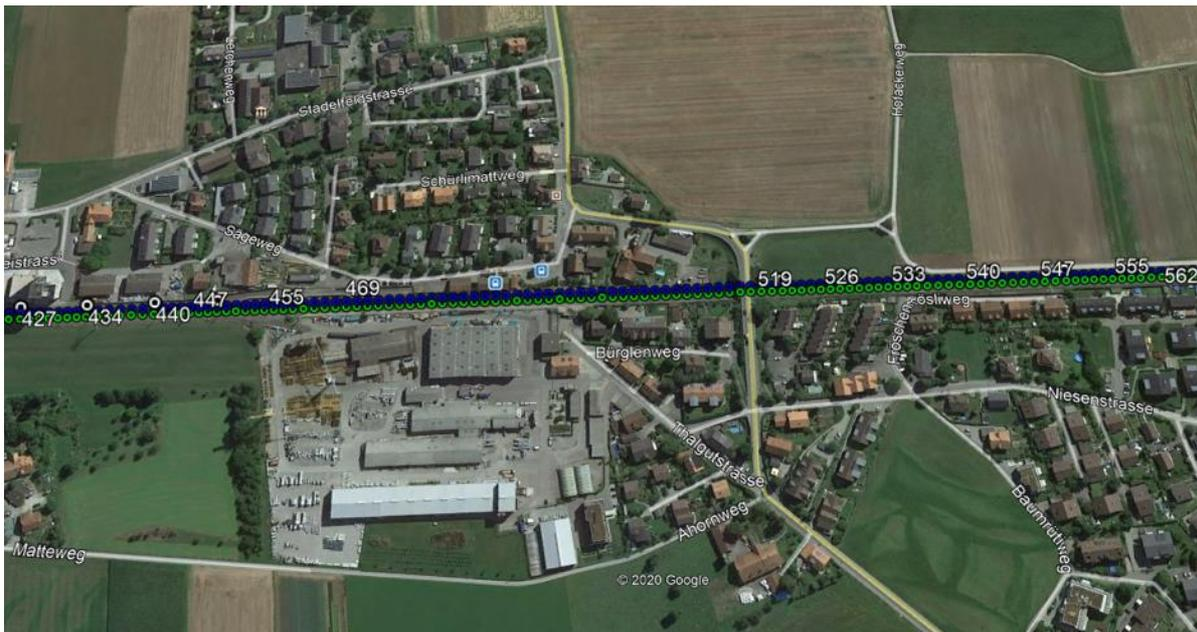
Figure 4-43 Google Earth picture showing the resulting mapping at station Wichtrach. Catenary masts are marked with white circles with their corresponding fiber channel. The green and blue circles mark the channel position on the track.
