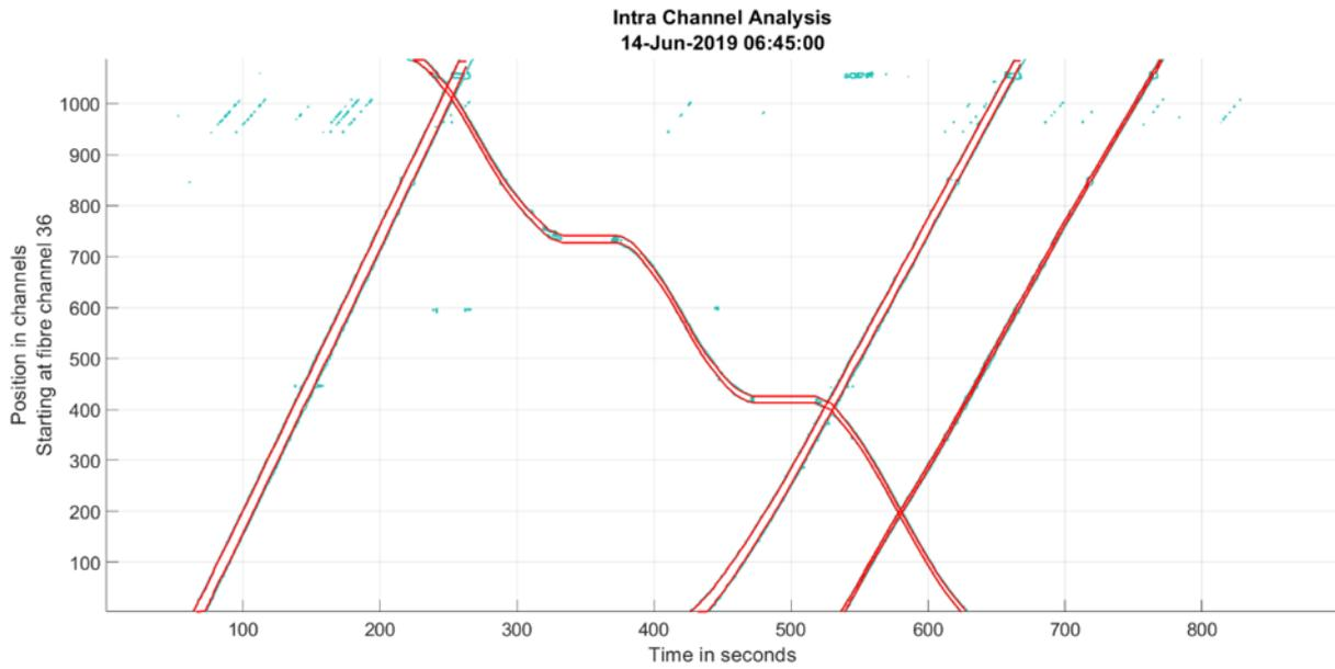
**Figure 4-47 Comparison between Intra and Inter Channel Analysis in a contour plot. The green lines represent the transition between noise and signal and the red lines show the achieved tracking of trains.**
