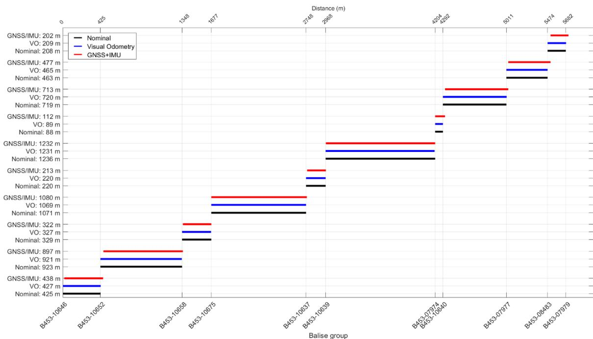
**Figure 6-3: The nominal distance (black) from DfA, the distance calculated by using the GNSS/IMU combined measurement (red) and the distance calculated by Visual Odometry (blue) are compared.**
