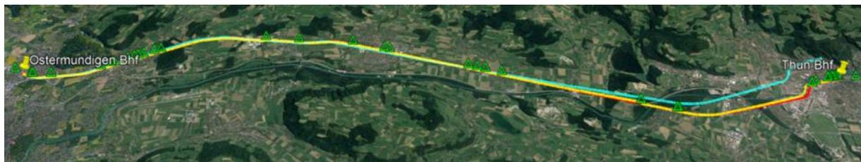
**Figure 6-14: The position calculated with the Visual Odometry (cyan) is corrected by using global reference like railway points (green triangles). The corrected position (yellow) is compared with the GNSS / IMU combination (red).**
