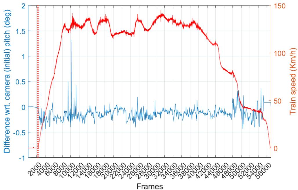
Figure 3-23: The difference (in blue) of the pitch measured during the whole measurement run, with respect to one measured during the calibration in the initial frames, where the train was at rest. In red, the train speed is displayed. The red dotted line highlights the frame when the train started.
