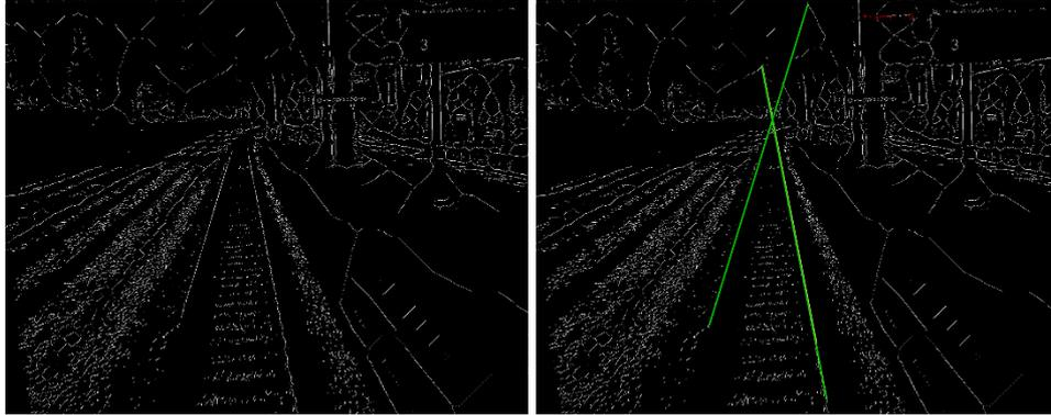
**Figure 3-16 (left):** Picture after iterative erosion and dilation, **(right):** Picture after applying the HoughLinesP line detection
