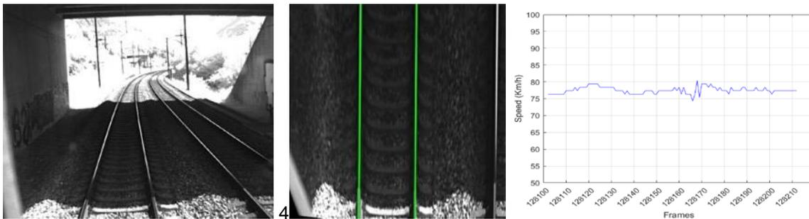
Figure 3-58 (left) Image collected from the camera, where a train is passing a short tunnel, (center) the image transformed to a bird-eye view where the railway track (green) can be identified, (right): the absolute speed is measured with precision meaning that the template matching is not affected by the shadow of the short tunnel.
