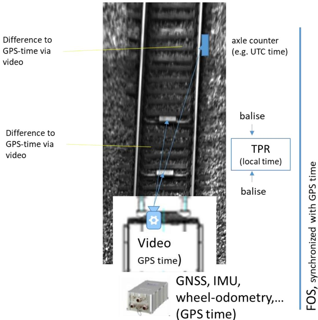
**Figure 6-1 - time synchronization and references for ground truth**
