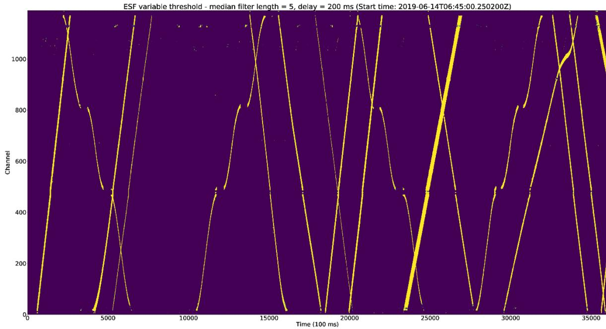
Figure 4-33: ESF threshold based on clustering with variable filtering for the 1 hour interval (14 June 2019)
