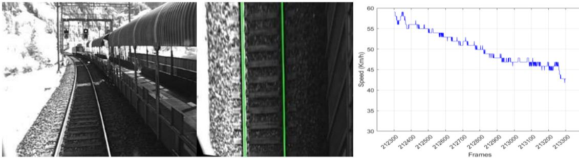
Figure 3-57 (left) Image collected from the camera, where a train is passing nearby causing shadow on the track, (center) the image transformed to a bird-eye view where the railway track (green) can be identified, (right): the absolute speed is measured with precision meaning that the template matching is not affected by the shadows.
