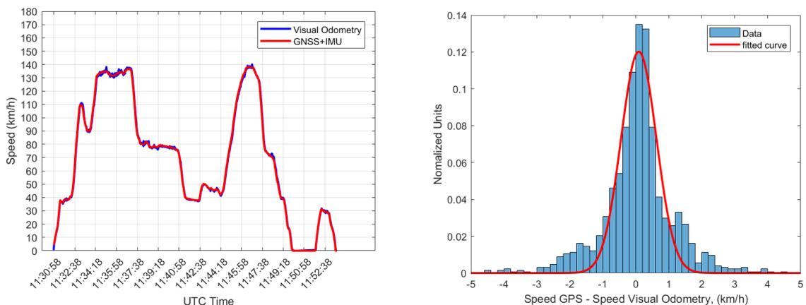
**Figure 6-8 (left)** The absolute speed measured with Visual Odometry (blue) is compared to the one measured with the combination of GNSS and IMU (red) during the drive OT\_4H. **(right)** The distribution of the speed difference between the one measured with GNSS combined with IMU and the one calculated with Visual Odometry is shown for drive OT\_4H.
