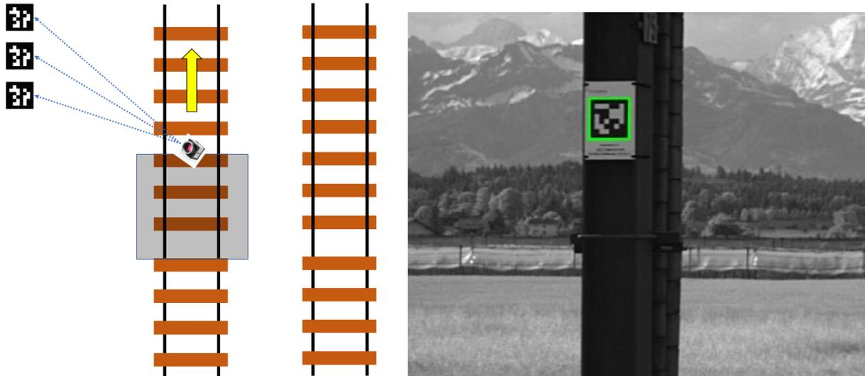
Figure 3-39 Left: scheme of the camera system moving forward and passing by an AprilTag. Right: image where the AprilTag is detected (green square).
