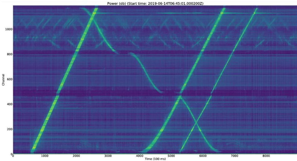
**Figure 4-8: Raw data power using a 500 sample (0.2 sec) window and a 250 sample (0.1 sec) step**
