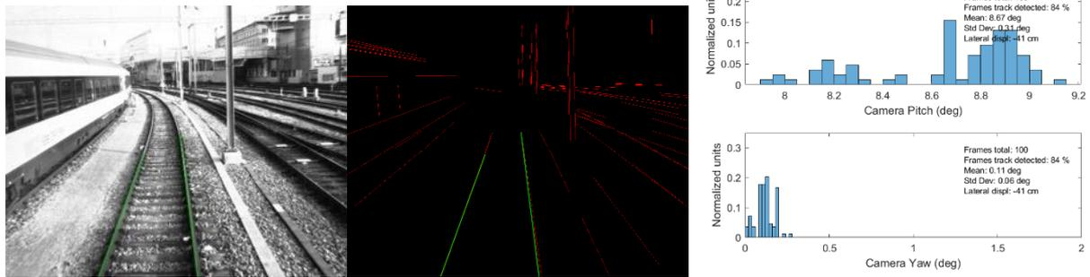
Figure 3-51: Left: Image collected from the camera with identified railway track (green). Middle: Image processed with detected lines (red) and identified railway track (green). Right: Estimated pitch (top) and yaw (bottom) distributions.
