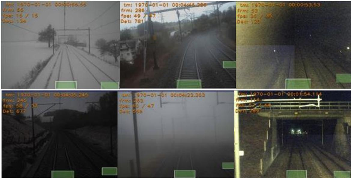
**Figure 7-7.** Examples of track detection at different lightings and environmental conditions (from top left to bottom right: snow, cloudy, tunnel, dusk, fog and night).
