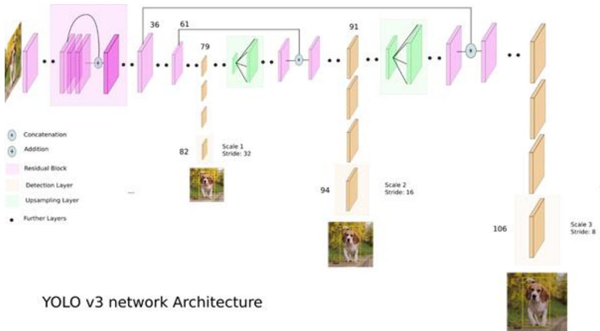
Figure 7-2. Schematic representation of the YOLO framework architecture.
