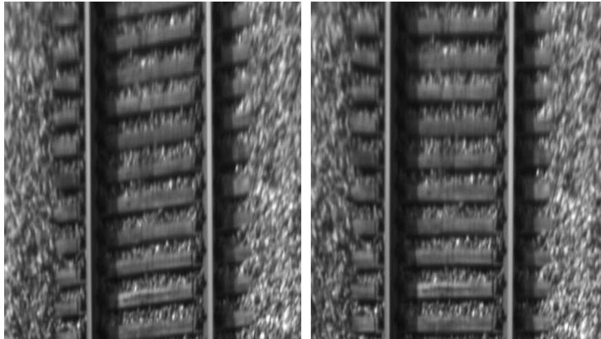
Figure 3-22 (left): The image rectified for pitch and yaw estimation and transformed to a bird-eye view. The sleepers are not parallel to the bottom of the image, meaning that the tilt shall be corrected, (right): By correcting the tilt of the camera, the sleepers are parallel to the bottom of the image.
