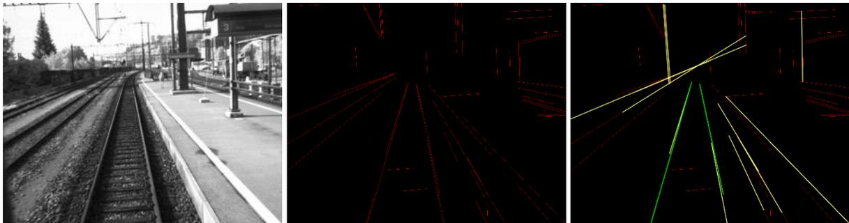
**Figure 3-17 (left):** Original picture, **(middle):** Segments found by the Fast line detector, **(right):** Lines found by the Fast line detector.
