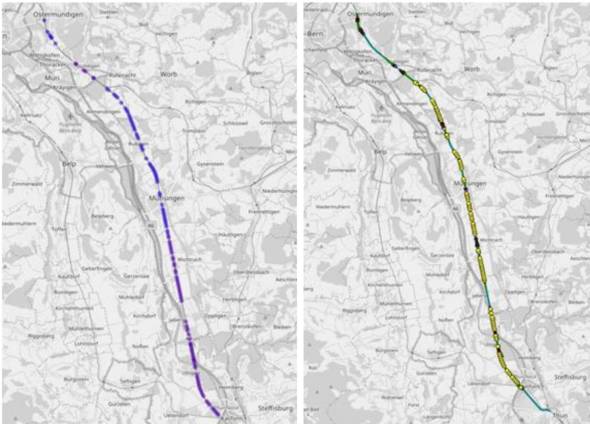
**Figure 7-13.** Analysis of recognized kilometer boards. **(left)** Recognized kilometer-boards along the route. **(right)** Traveled track sections extracted from the DfA (ground truth).
