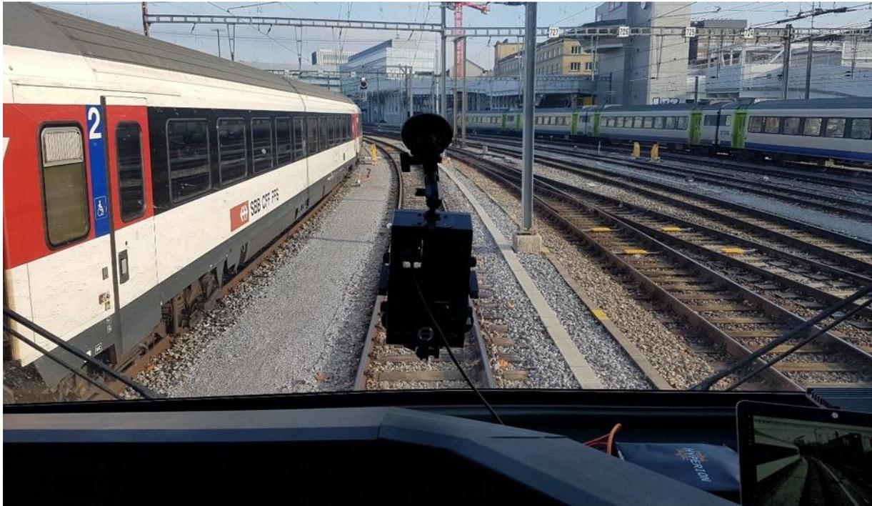
Figure 3-3 The camera box mounted on a RABDe 500, during the run from Biel to Lausanne.
