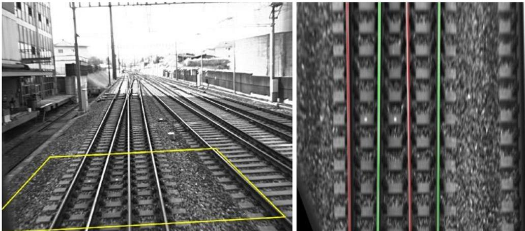
**Figure 3-24 (left):** A region of interest of 6x6 meters is defined in the collected raw image, **(right):** the region of interested is rectified and transformed according to a bird-eye view and the main track (green) and a side track (red) are identified.
