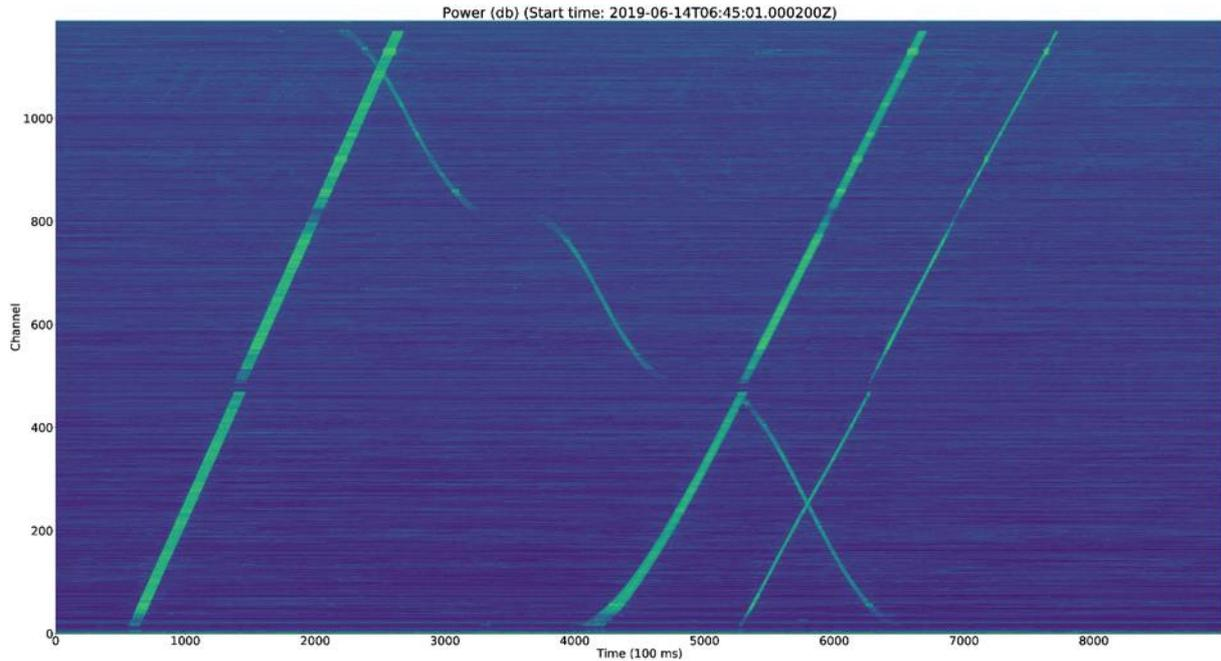
Figure 4-24: Welch PSD (db) estimate 500 (3 x 250 + 125) x 250 (hann) from 120 to 400 Hz
