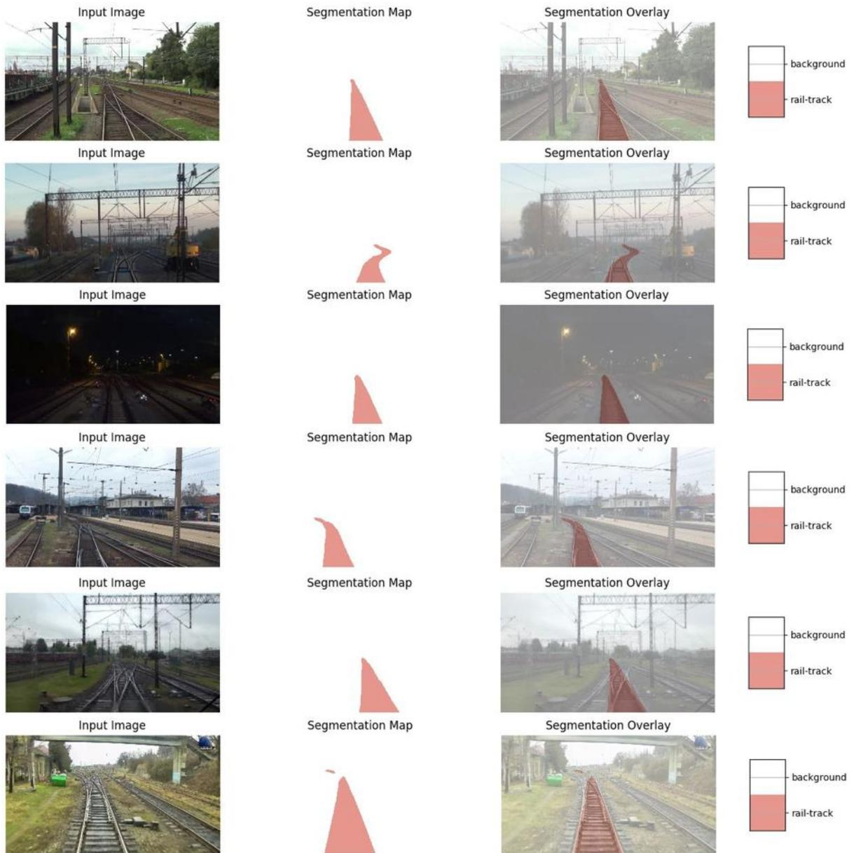
Figure 7-15. Example images showing the semantic segmentation of the predicted route.
