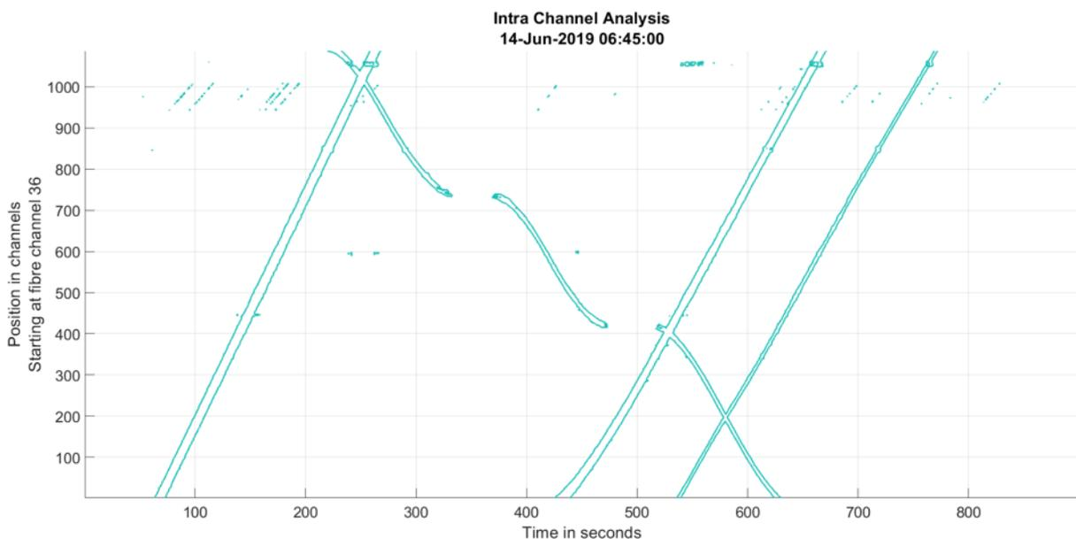
Figure 4-46 Results of the Intra Channel Analysis represented as a contour plot. The green lines show the transition between noise and signal.
