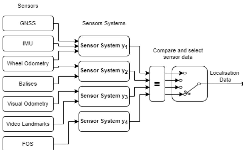
Figure 5-1: Example of a x-out-of-y system architecture
