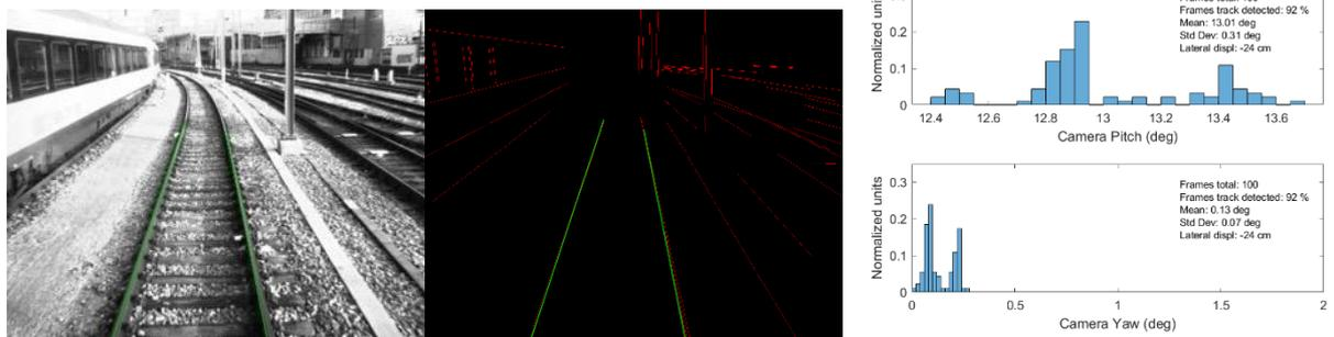
Figure 3-53: Left: Image collected from the camera with identified railway track (green). Middle: Image processed with detected lines (red) and identified railway track (green). Right: Estimated pitch (top) and yaw (bottom) distributions.
