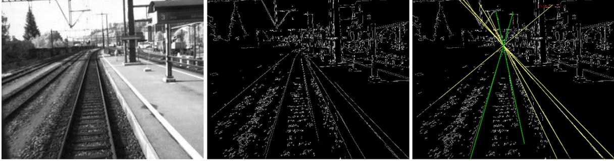
Figure 3-14 (left): Original picture, (middle): Picture after Canny contour detection, (right): Picture after HoughLinesP line detection
