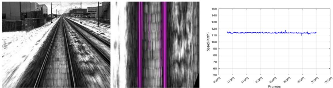
**Figure 3-56: (left)** Image collected from St Gallen to Bern with little snow on the railway track. Motion blur can be observed due to low illumination of the scene and high speed of the train, **(center)** the image transformed to a bird-eye view where the railway track (magenta) is difficult to be identified, **(right):** the absolute speed is measured with precision meaning that the template matching is not affected by the snow and by the motion blur.
