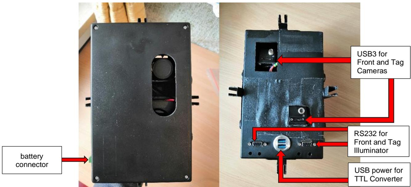
**Figure 3-2 Front and Back view of the camera box**
