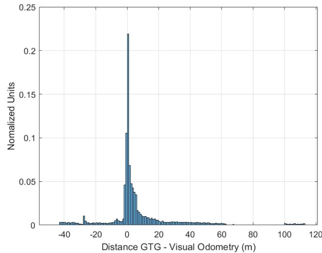
**Figure 6-17** The distribution of the difference between the position measured from the GTG and the one calculated with Visual Odometry.
