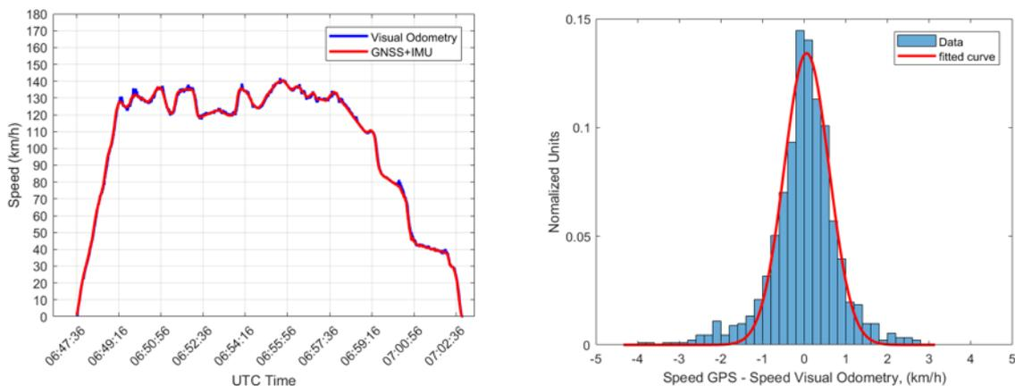
**Figure 6-5 (left) The absolute speed measured with Visual Odometry (blue) is compared to the one measured with the combination of GNSS and IMU (red) during the drive OT\_1H. (right) The distribution of the speed difference between the one measured with GNSS combined with IMU and the one calculated with Visual Odometry is shown for drive OT\_1H.**
