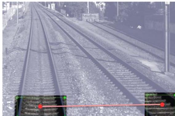
Figure 7-1. Example image of tracks detected using an object-based detector.
