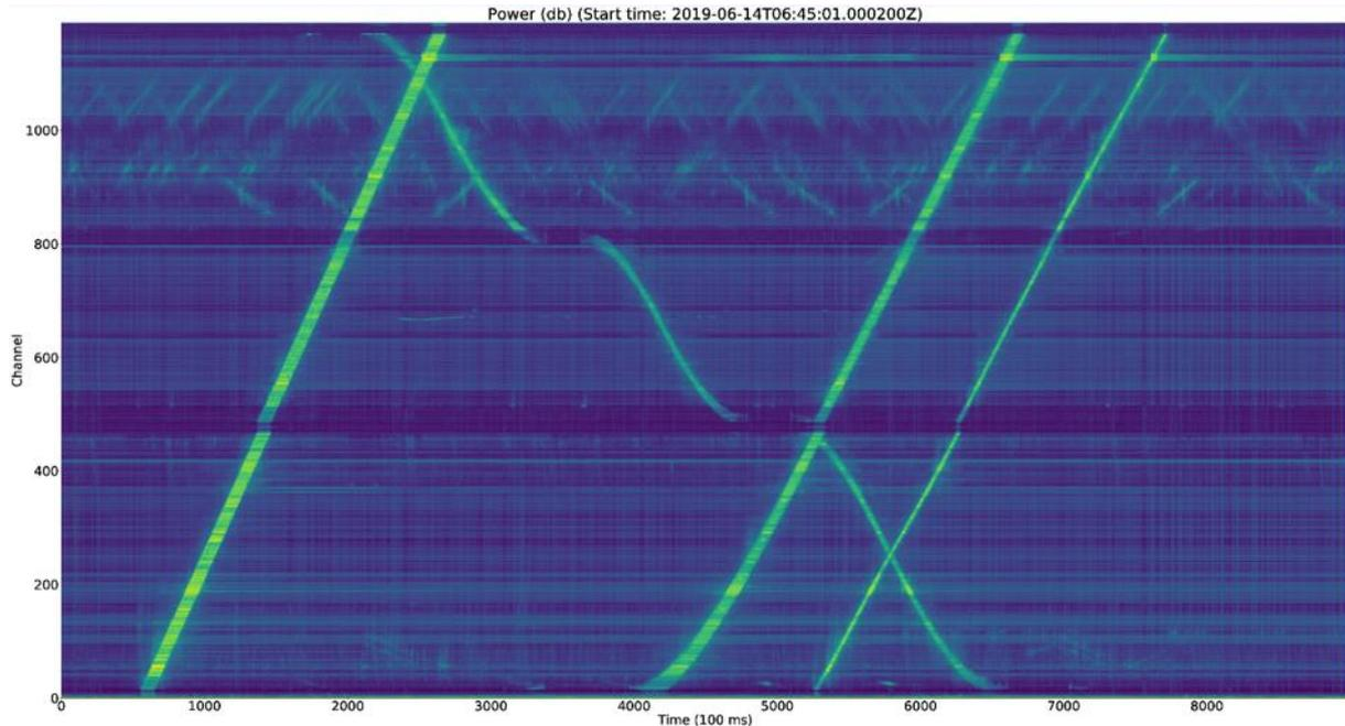
**Figure 4-7: Raw data power using a 2500 sample (1 sec) window and a 250 sample (0.1 sec) step**
