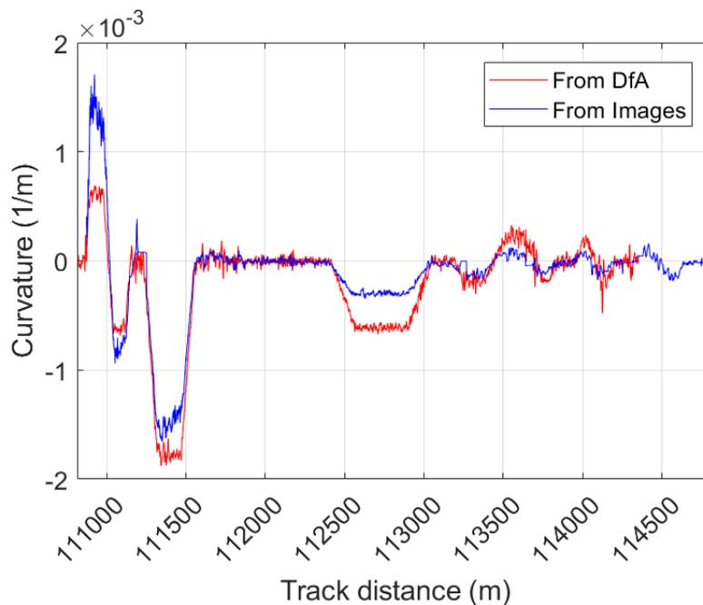
Figure 3-28 The estimated curvature, derived from the position of the railroad track in the image, is compared to the curvature stored in the database for a small section.
