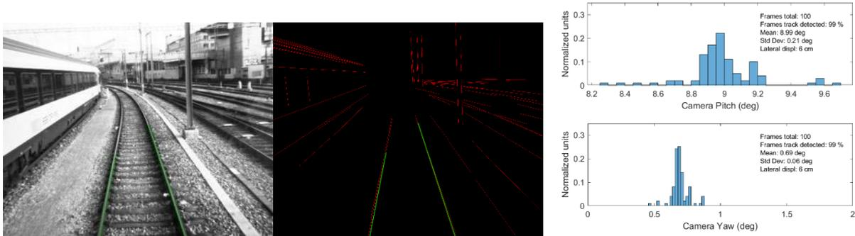
Figure 3-43 Left: Image collected from the camera with identified railway track (green). Middle: Image processed with detected lines (red) and identified railway track (green). Right: Estimated pitch (top) and yaw (bottom) distributions.
