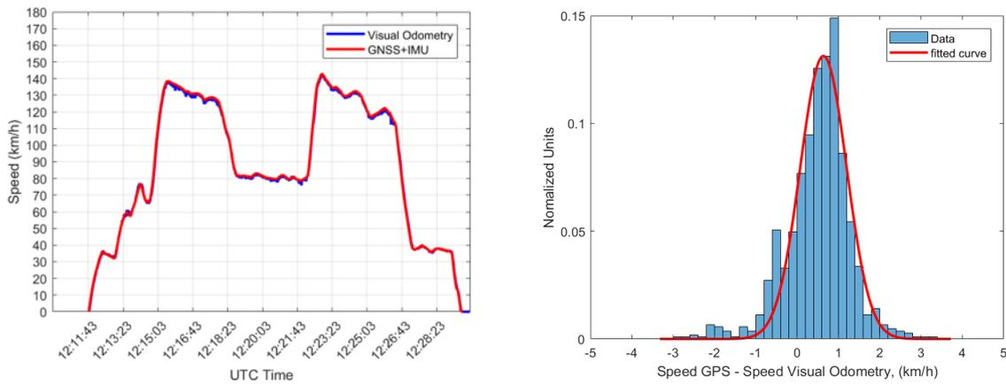
**Figure 6-12 (left) The absolute speed measured with Visual Odometry (blue) is compared to the one measured with the combination of GNSS and IMU (red) during the drive OT\_4R. (right) The distribution of the speed difference between the one measured with GNSS combined with IMU and the one calculated with Visual Odometry is shown for drive OT\_4R.**
