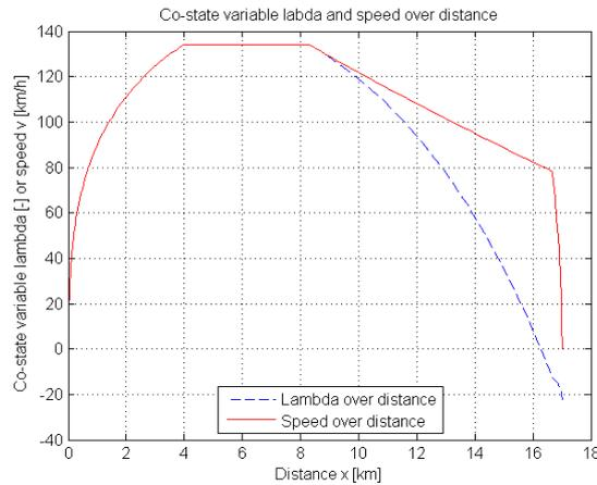
Figure 7: Co-state variable  $\lambda$  and speed over distance
