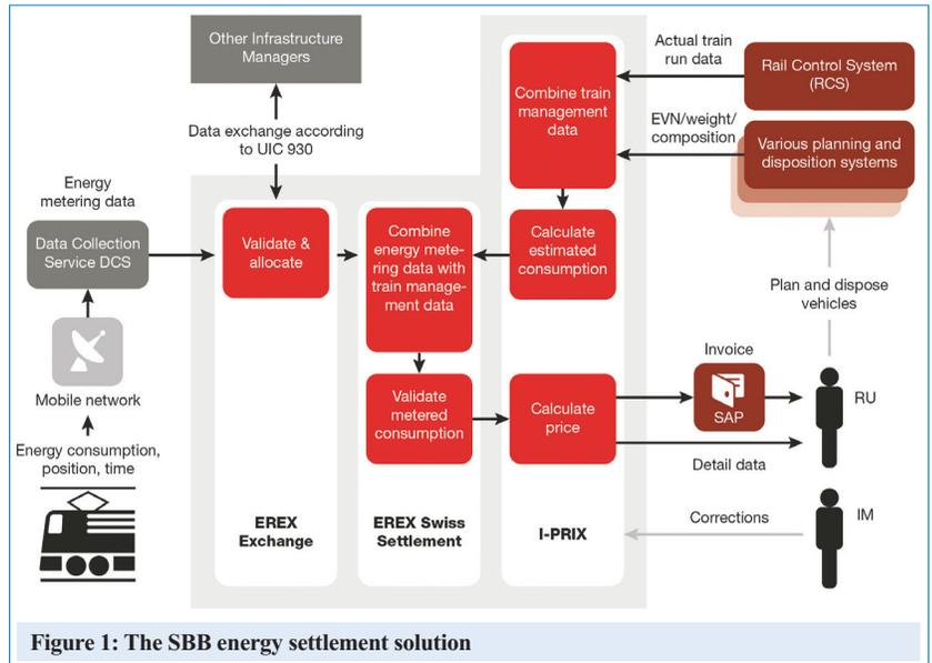
Figure 1: The SBB energy settlement solution
