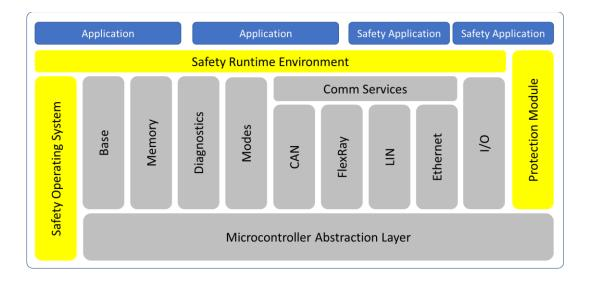
Figure 38: AUTOSAR SW Architecture with safety BSW
