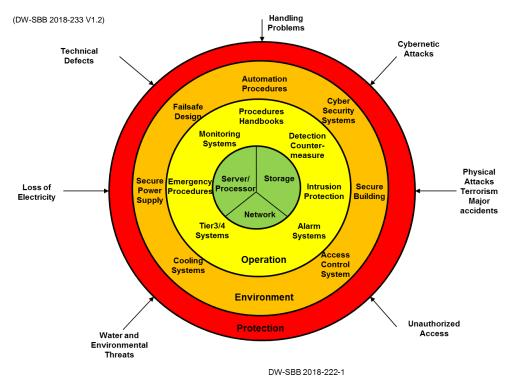
Figure 8: The shell model of a data center
