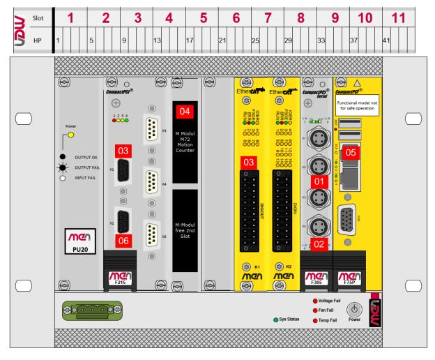
Figure 5 Onboard Unit (incl. identification of used Interfaces)
