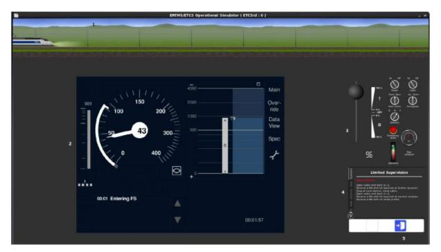
Figure 19 Operational Simulator standard execution user interface
