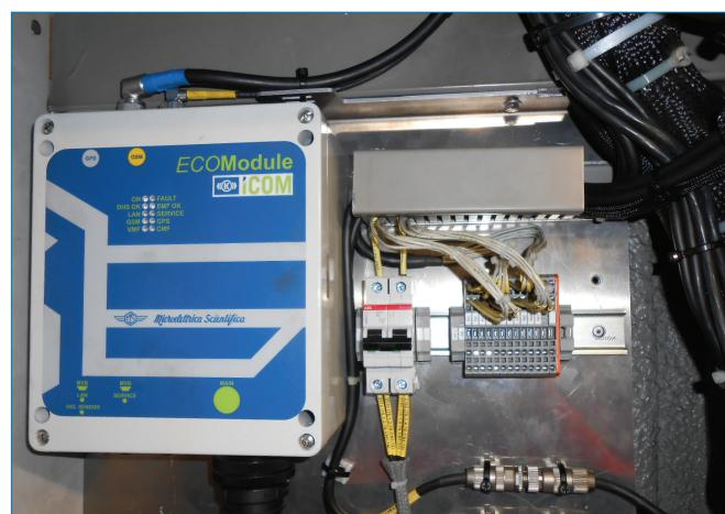
Figure 3: Installed energy measurement device on-board a Re450
