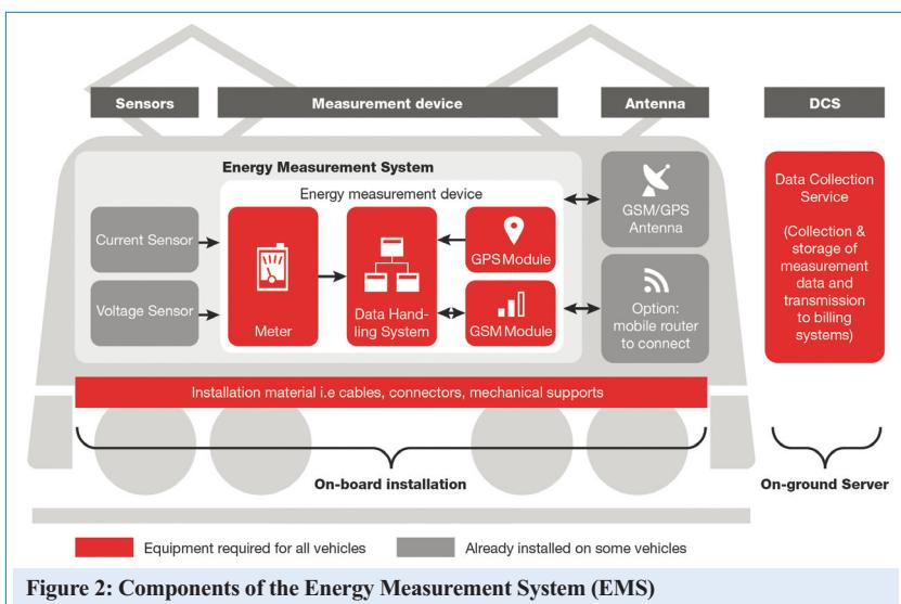
Figure 2: Components of the Energy Measurement System (EMS)
